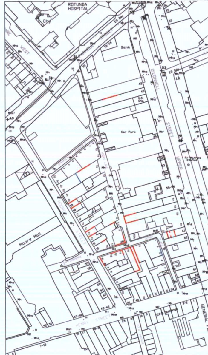
Fig. 4 Map of study area identifying walls subject to forensic investigation in RED.
