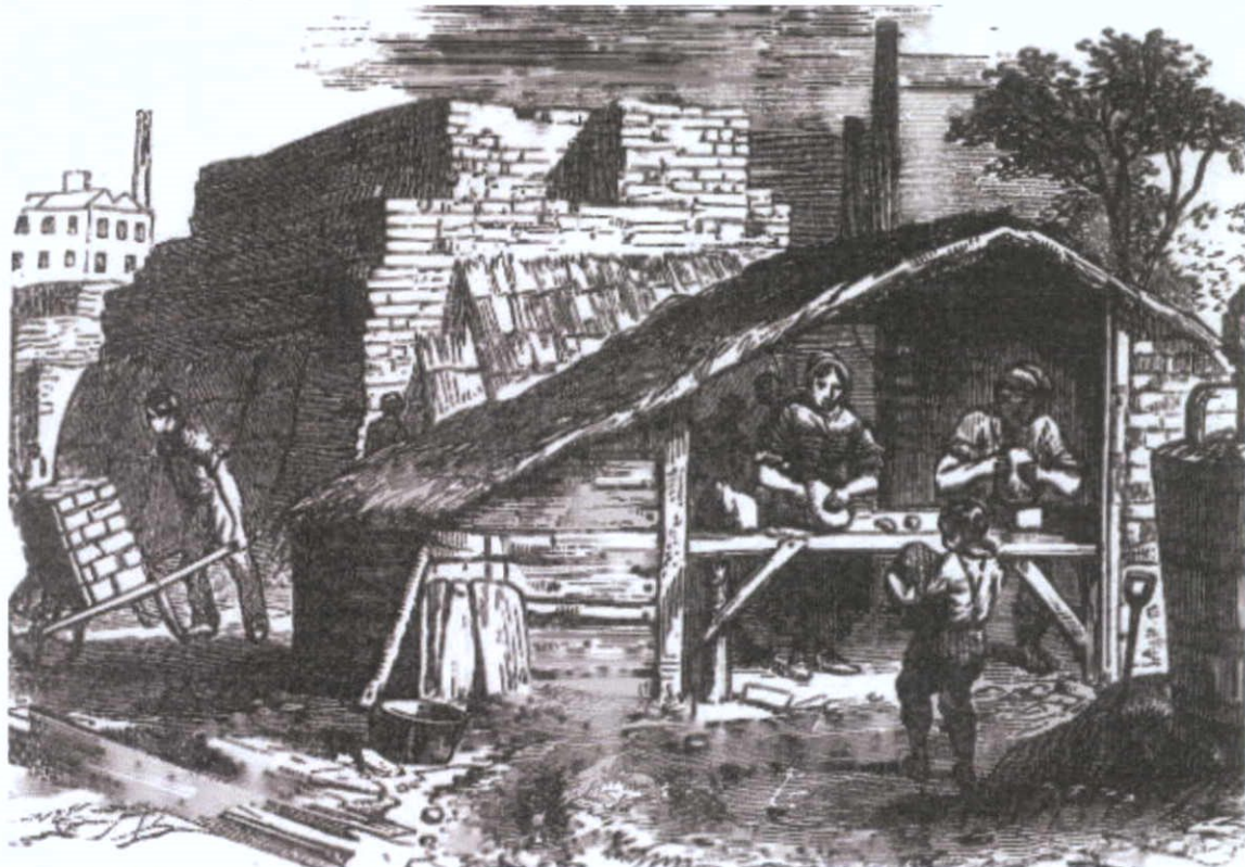
Fig.3.3: A brickyard depicted in ‘The Boy’s Book of Trades in 1871 showing a man and woman (possibly husband and wife) moulding bricks at a bench in a rough timber shelter, while a small boy (possibly their son) carries clay from a pug mill with the circular track walked by the horse also seen. In the background, a part-dismantled clamp can be seen, with a man wheeling bricks on a barrow.
