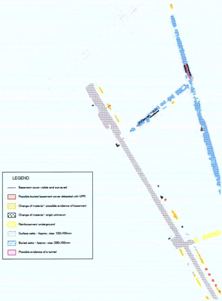
P 49 The GPR survey of the internal street network, indicating existence of setts below tarmac surfaces. Please Note, due to their concealed presence, it is not possible to confirm the extent of disturbance to accommodate extensive ground works in the past. Source:Murphy Geospatial fix image
