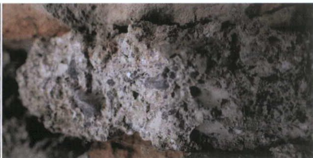
Fig.5.1.13: Poorly sorted bedding mortar containing limestone, chert and quartz aggregate.
