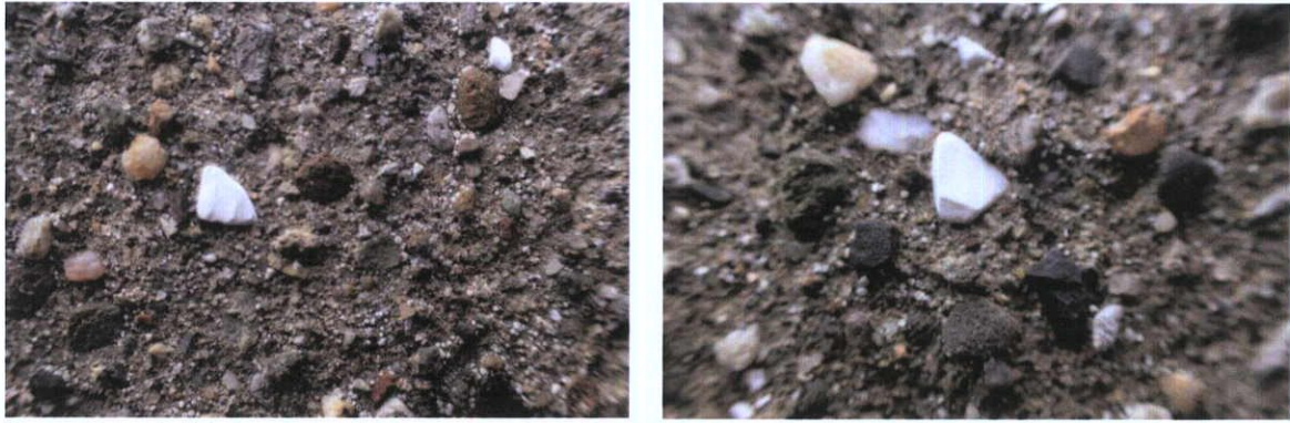
Fig.4.10.4: Shell forms a significant proportion of the aggregate, indicating the use of a beach sand.
