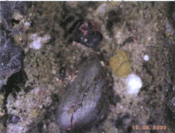
Fig. 4.17.8: Rounded limestone and crushed yellow brick aggregate
