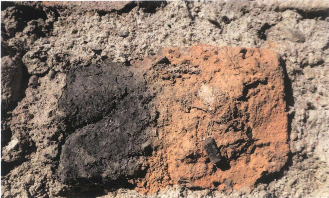
Fig.5.3.19: Partially overburnt clamp fired brick with angular limestone inclusions, some partially calcined.
