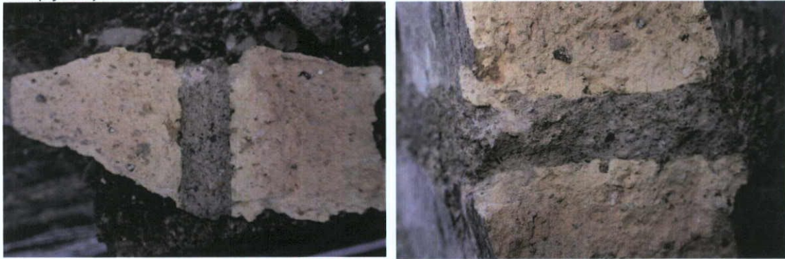
Fig.5.2.8: Cross section showing the 1920s brick with natural stone inclusions in an evenly-fired matrix and bonded with a cementitious bedding mortar. Sample #90.
