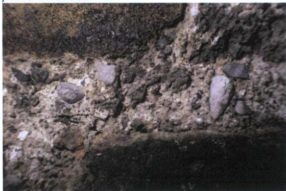
Fig.4.4.7: Coarse-grained limestone, quartz and chert with brick pozzolan and lime lumps.
