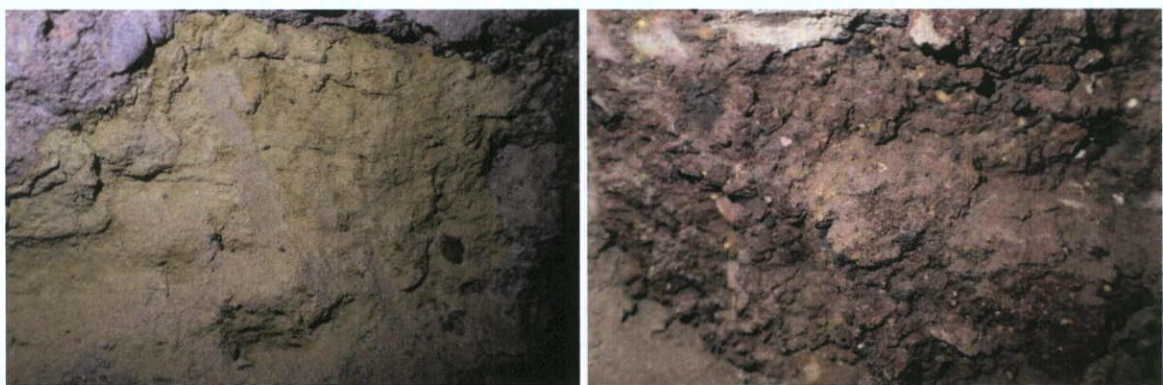
Fig.5.2.18: Detail of the fine-grained yellow stock brick from the 1920s (left) and the dark-red clamp-fired Georgian brick which contains abundant natural stone inclusions, partially calcined limestone and burnt 'hot spots' suspended in the matrix.
