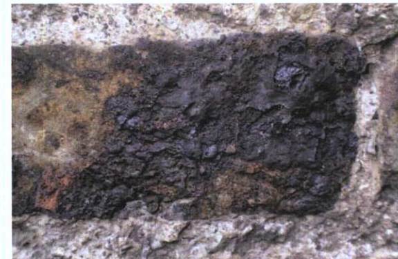
Fig.4.4.7: Coarse-grained limestone, quartz and chert with brick pozzolan and lime lumps.
