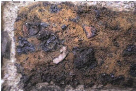
Fig.4.4.5: Overburnt clamp-fired yellow stock brick showing calcined stone and vitrified zones.
