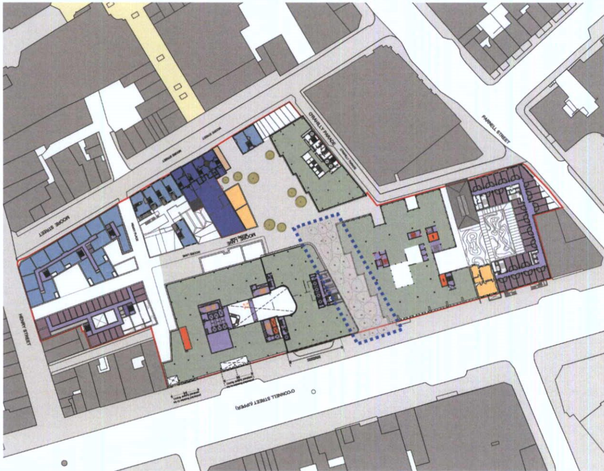
Figure 4.2: Iteration of the Masterplan from July 2020 showing the inclusion of a canopy within the New Street proposed between O’Connell Street and Moore Street – outlined by a blue dashed line (Overlay by SLA).
