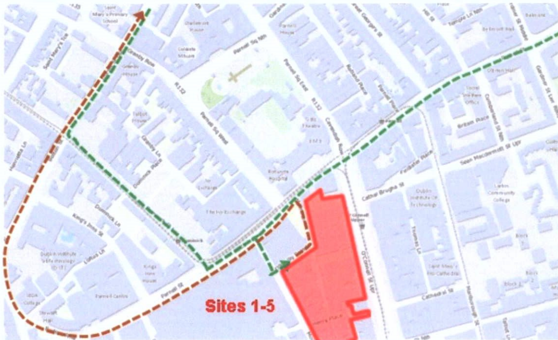
Figure 13.23: Emerging Haul Routes for Construction Traffic (Inbound in green and outbound in red).
