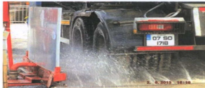
Figure 9 – Typical Wheel Washing Facility
