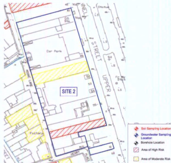
Figure 46 – Site 2 areas of Potential Contaminated Material
