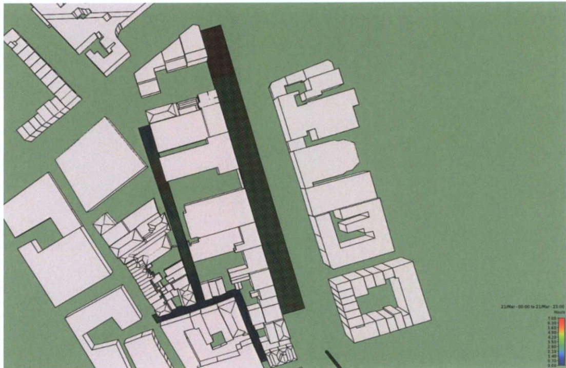
Figure 10.6: Sunlight Exposure on O'Connell Street, Henry Place & Moore Lane, March 21 st (Baseline Site).
