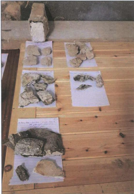
P 19 Samples of mortar collected on site by Dr. Jason Bolton for analysis.
