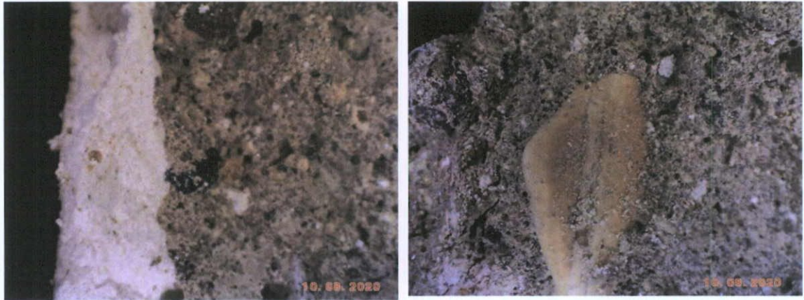
Fig.4.8.6: Microscope cross-section of the internal plaster of No.4 Moore Street, with coarse shell fragment.
