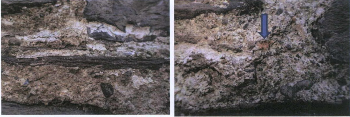
Fig.6.4.6: Slate pinnings (left) and coarse brick aggregate (right, arrowed) as an occasional component of the aggregate fraction of the mortar.
