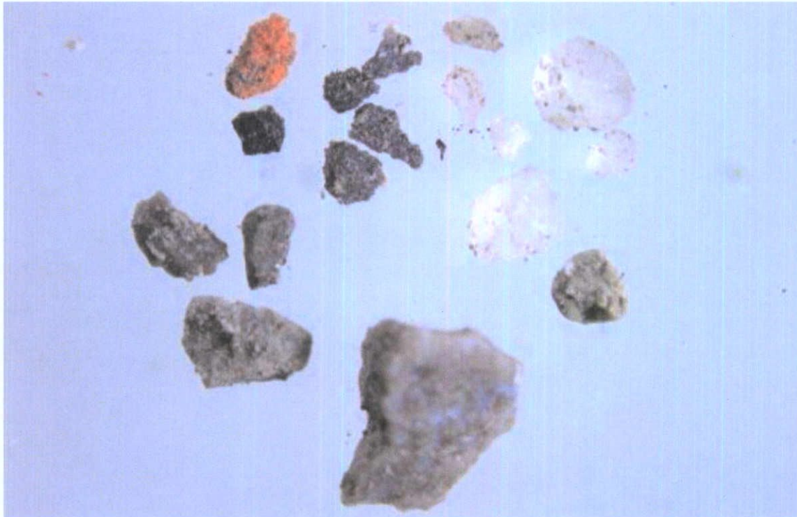
Fig.4.16.26: In contrast, the aggregate of the lime-based bedding mortars consists mainly of limestone, quartz, some chert and a fraction of brick aggregate.
