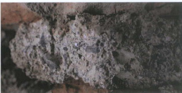
Fig.5.1.13: Poorly sorted bedding mortar containing limestone, chert and quartz aggregate.
