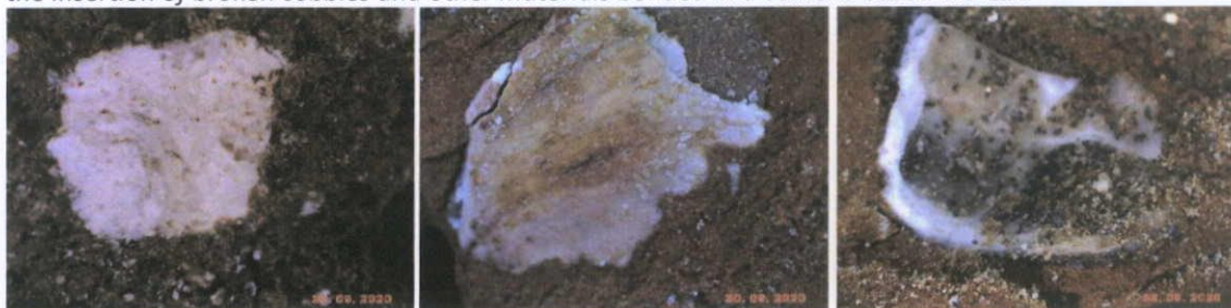
Fig.5.3.8: The late eighteenth/early nineteenth century mortars contain abundant lime limps (left) but no obvious porous brick aggregate or pozzolanic brick dust; while a proportion of the brick contain shell fragments as inclusions within the matrix – these are partially fired indicating that they were contained within the brick during manufacture.
