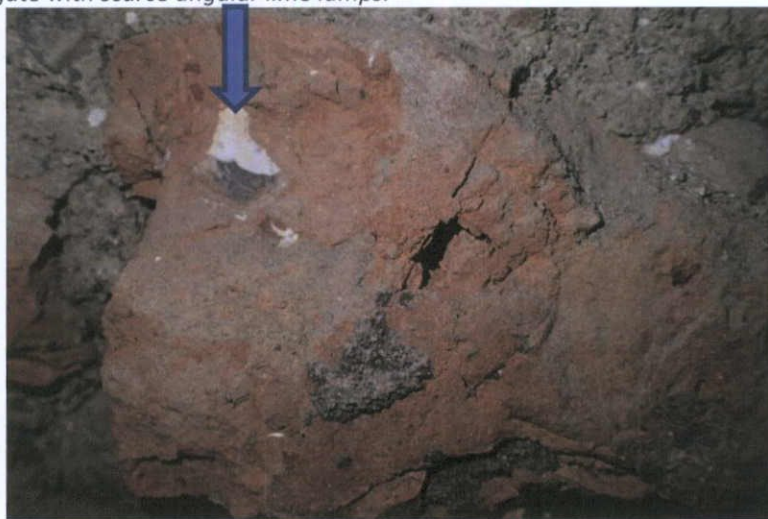
Fig.6.1.6: Shell (arrowed), partially fired, inclusion within the brick.
