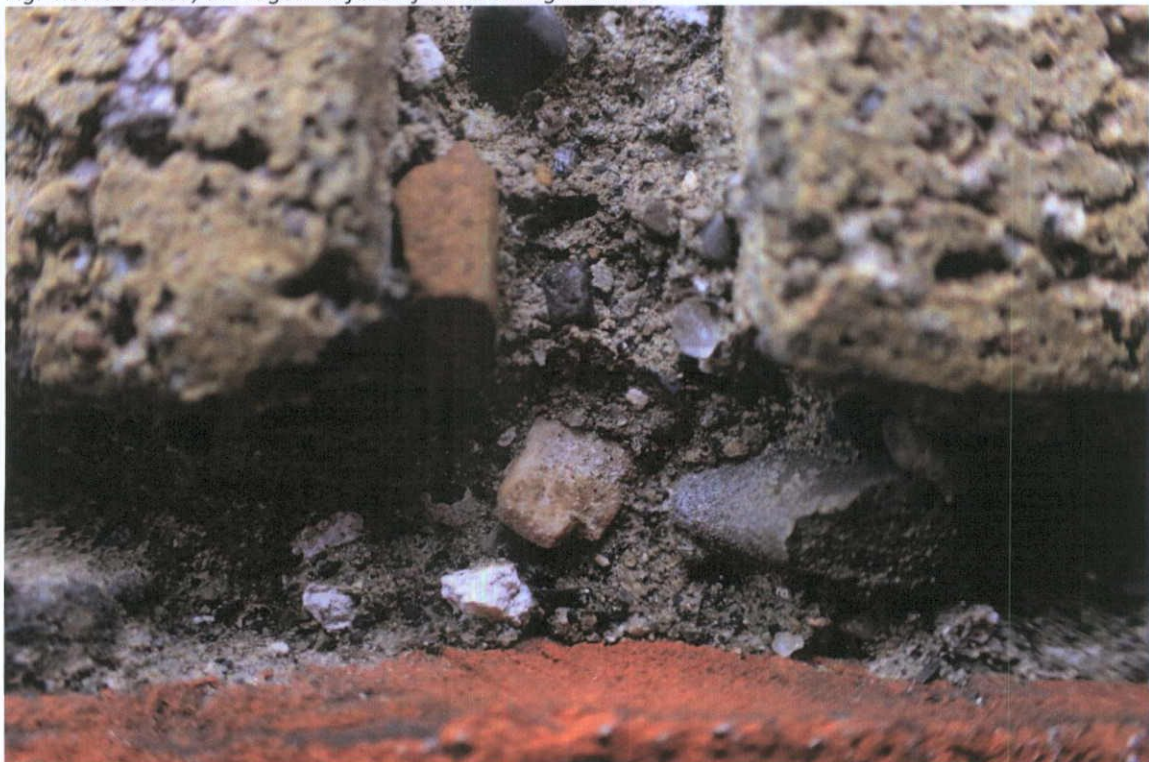
Fig. 4.17.4: Poorly sorted limestone, sandstone, quartz and chert aggregate with coarse lime lumps in a water-damaged lime binder.
