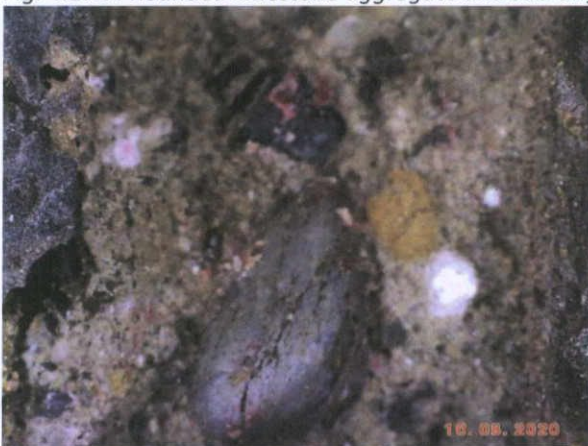
Fig. 4.17.8: Rounded limestone and crushed yellow brick aggregate
