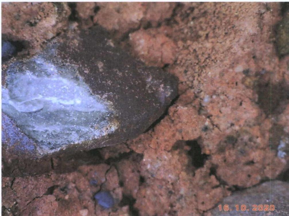
Fig.4.3.15: Microscopic detail of the core of a brick, likely to originate from the Moore Street brickfield. The brick contains poorly sorted and often partially calcined limestone and fine quartz.
