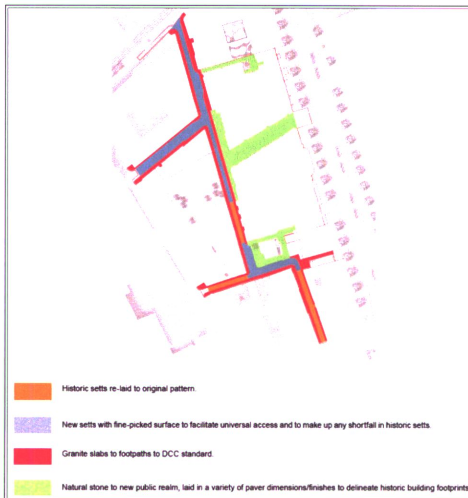
Figure 18.7: Indicative location for the re-laying of the historic setts in the public realm
