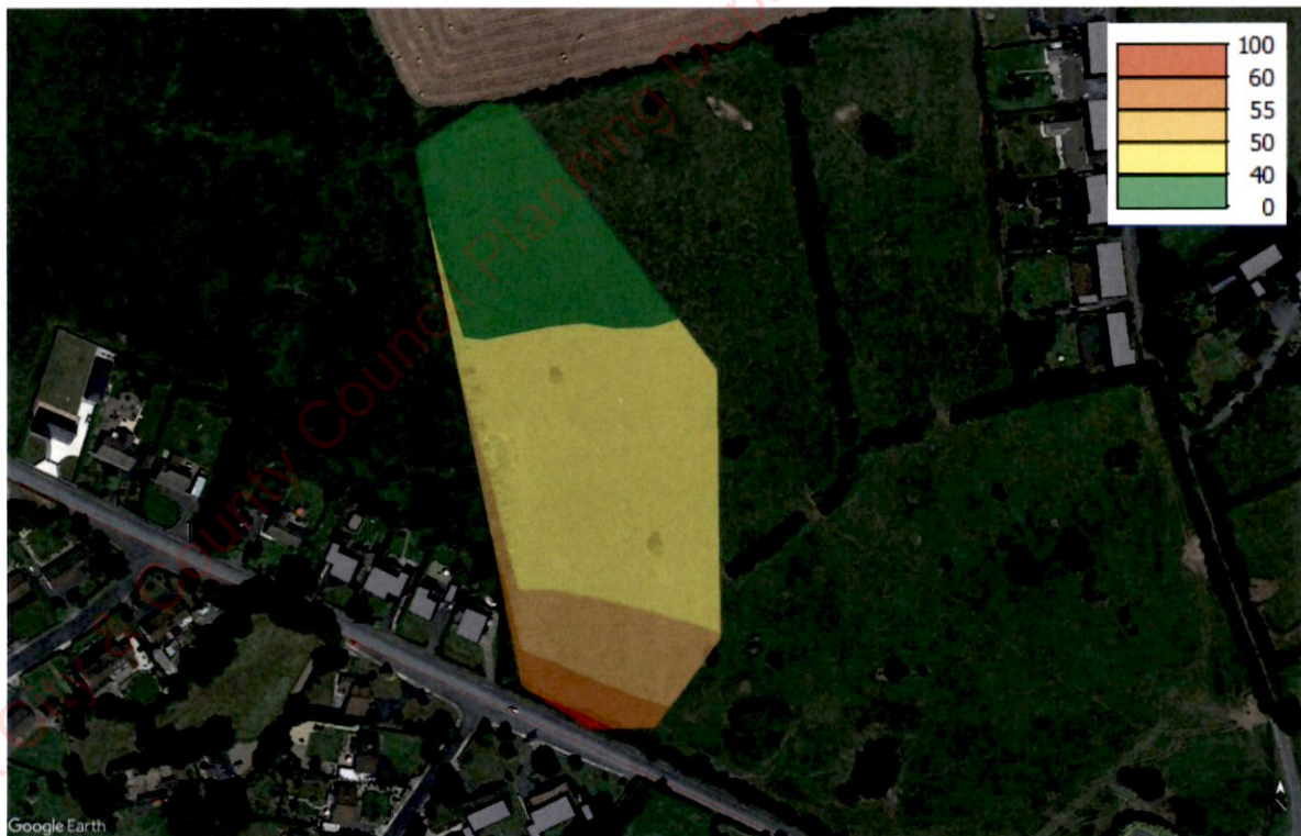
Figure 11.9 Initial Noise Risk Assessment – Night time (4m height)
