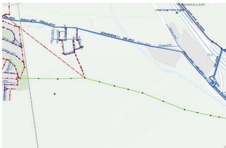
**Figure 3.7:** Irish Water infrastructure adjacent to application site, extract from enclosed Confirmation of Feasibility
