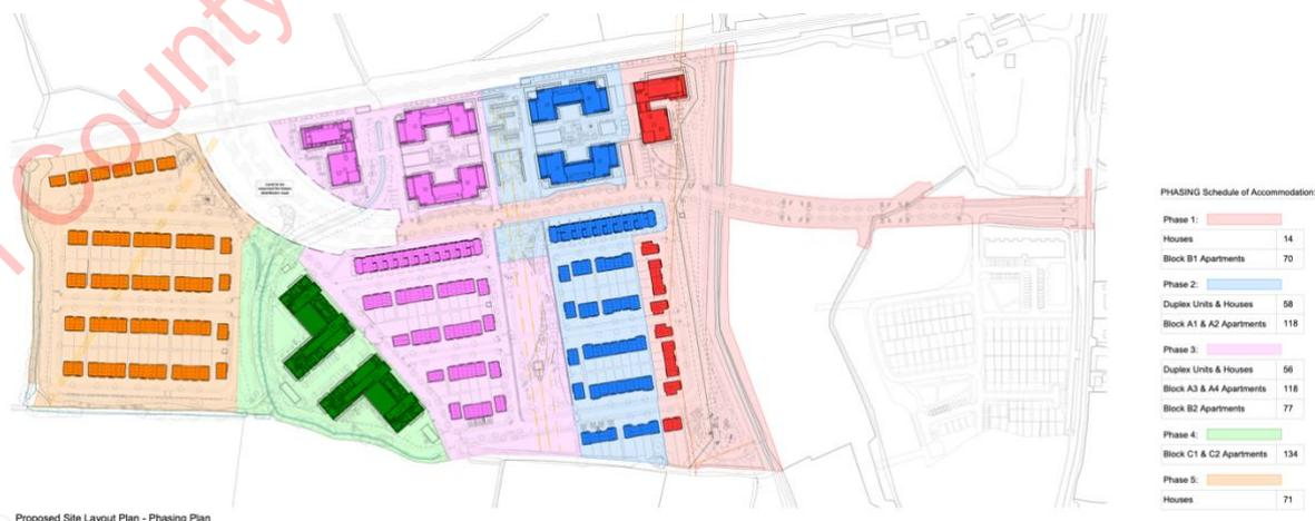
**Table 3.5: Proposed Construction Phasing Plan**
