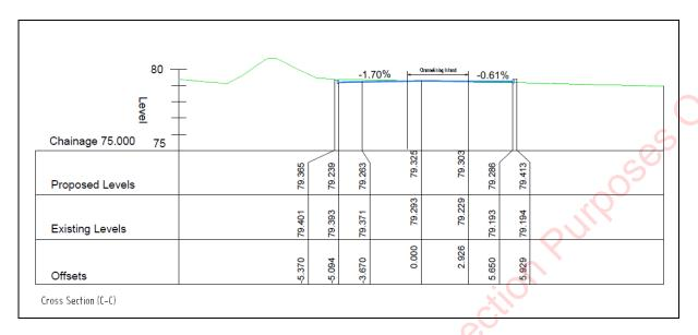
Figure 4: New kerbs and shallow crossfall on cross section south of channelising Island
