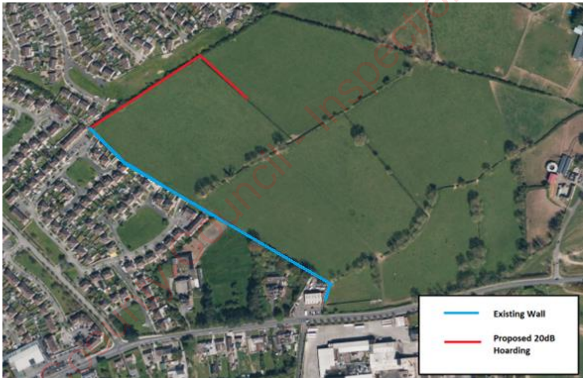
Figure 8.1: shows locations and type of hoarding required
