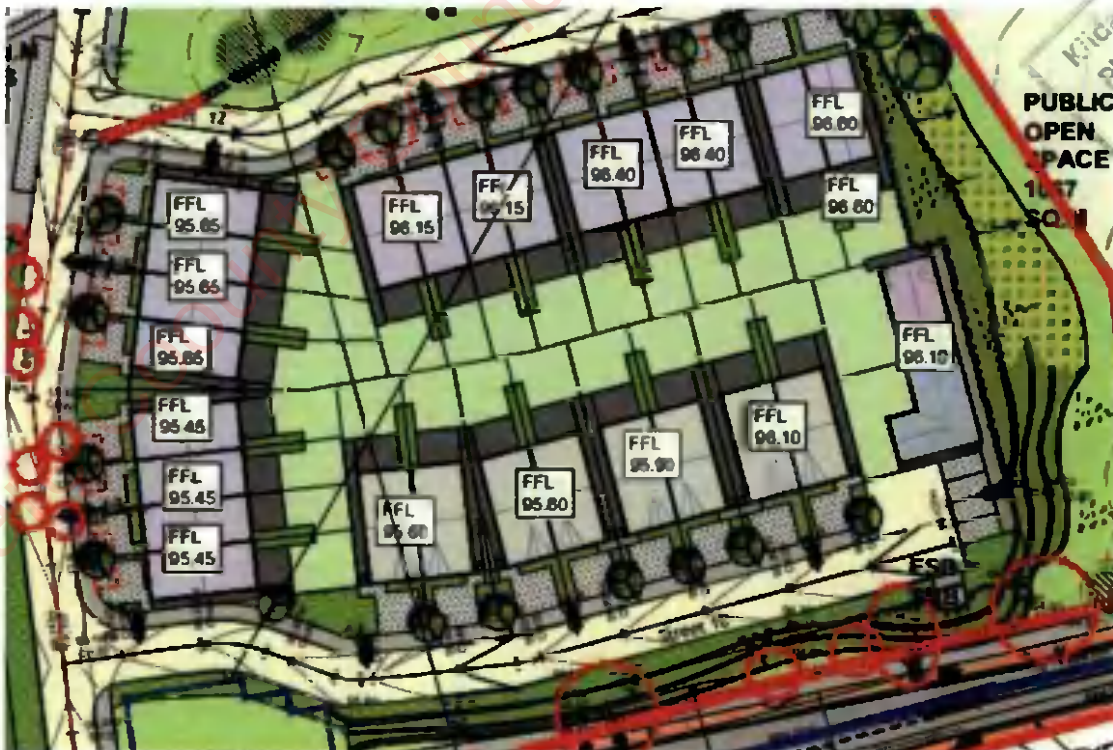
Figure 2.9: Current proposed gardens showing bioretention areas
