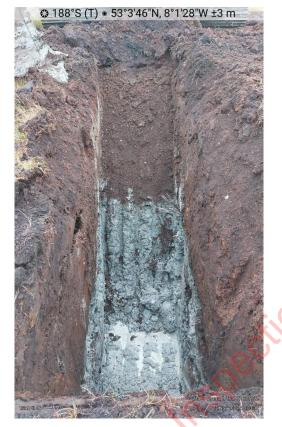
Figure 2-2: Photo of TP06 through peat and underlying cohesive glacial till close to the Turbine 5 foundation location.
