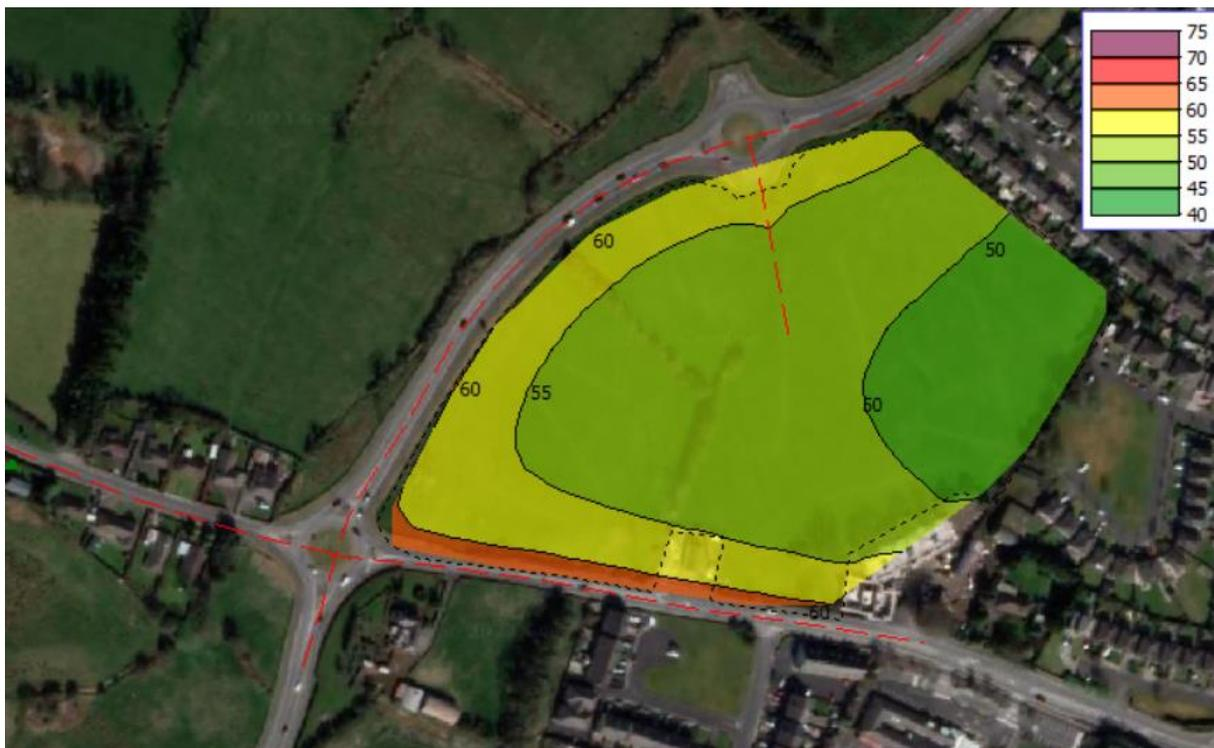
Figure 9.9 Night-time noise contours in dB(A) over existing site – in the absence of the development
