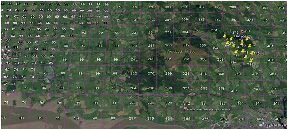
As you can see the guide (IFP) elevation which does not affect the IFPs, is exceeded for many of the proposed turbines. This does not mean that this is not acceptable. It does however require an IF assessment to be carried out by a certified IFP designer to assess possible impacts. When you're ready to engage on this I can advise on which companies are certified for this work. The result should confirm no impact, or recommend mitigations, e.g. lowering of some turbines elevations possibly
