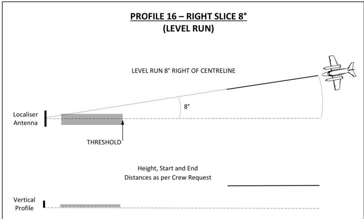
**Figure 5.7 – Right Slice 8° Flight Profile**
