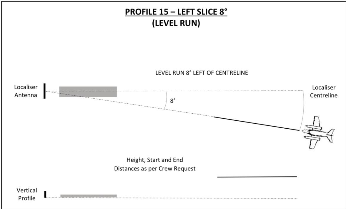
**Figure 5.6 – Left Slice 8° Flight Profile**
