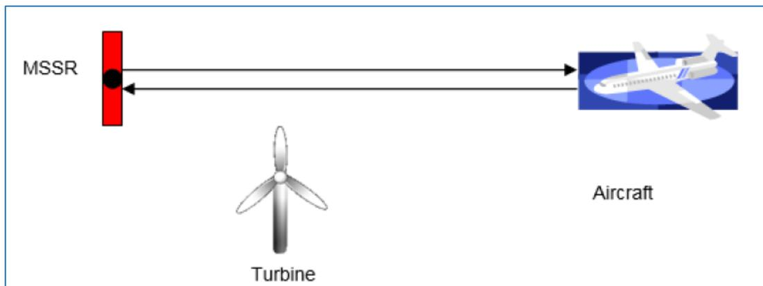
Figure 7: Direct interrogation and reply pulses
