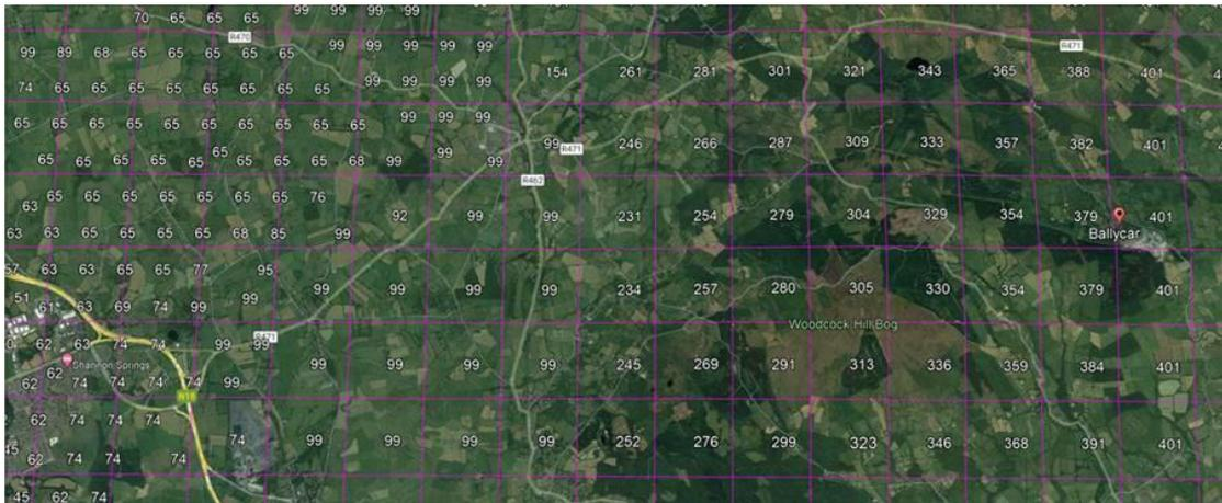
The values each grid cell represent an Above Mean Sea Level (AMSL: Site elevation + Height of obstacle) elevation value, above which, an IFP impact assessment will be required. In the case of the Ballycar area and taking the highest turbine height supplied, 254m added to an approximate site elevation of 240m, gives an AMSL elevation of in excess of 400m, which is above the safeguarding values in this area.
