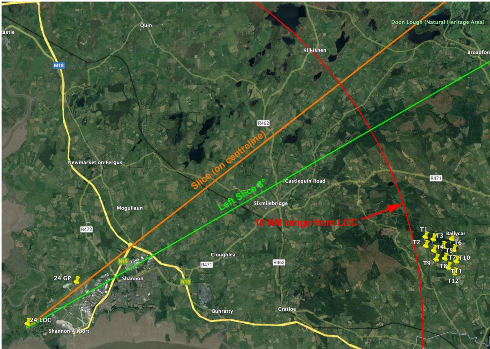
Figure 6.4 – Slice and Left Slice 8° Tracks
