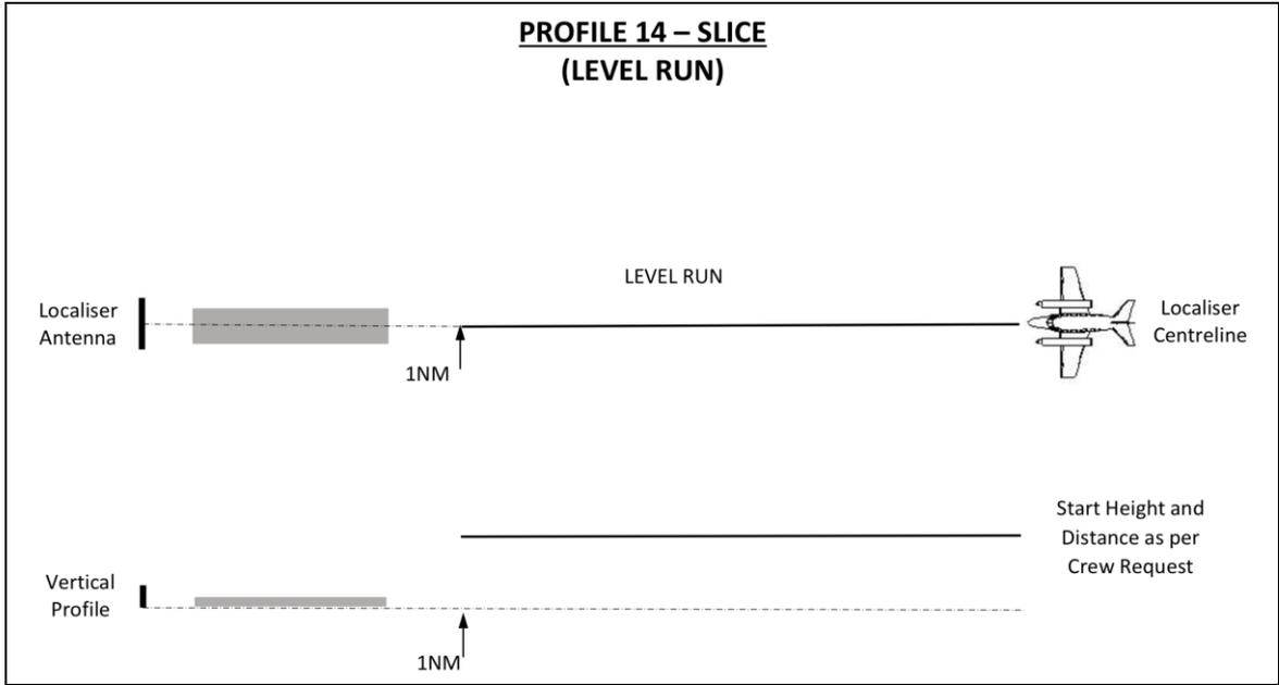
**Figure 5.5 – Slice Flight Profile**
