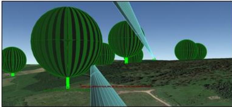
Figure 14. 3D View of T07 relative to nearest radio links
