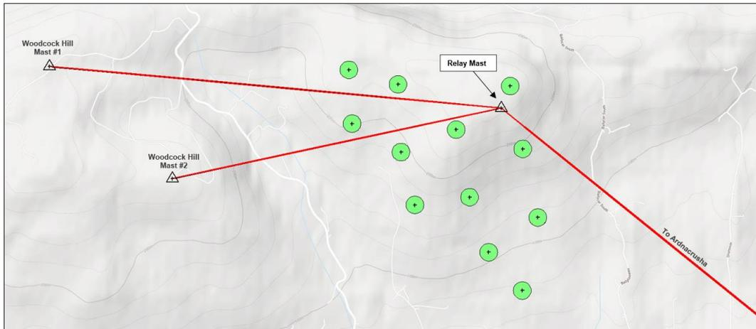
Figure 31. Proposed Relay Mast Location and relay links to Ardnacrusha
