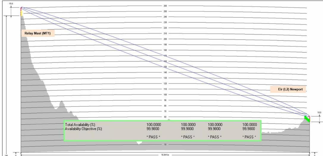
Figure 23. Relay Mast – Newport Path Profile
