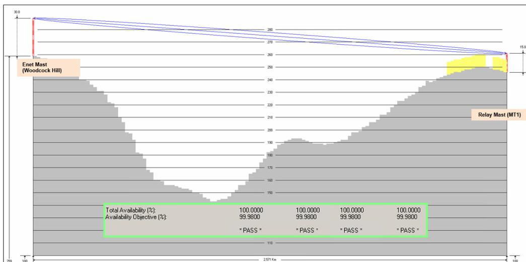
**Figure 10. Woodcock Hill – Relay Mast Path Profile**
