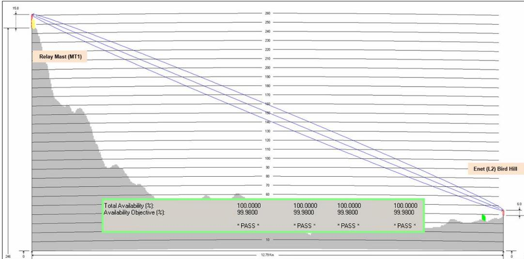
Figure 11. Relay Mast – Birdhill Path Profile
