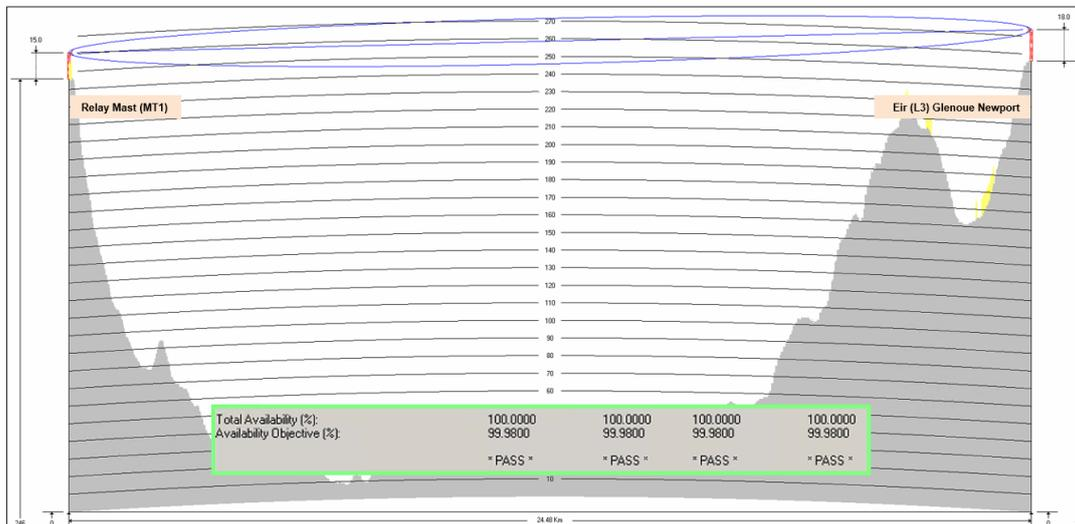
Figure 24. Relay Mast – Glenoue Newtown Path Profile
