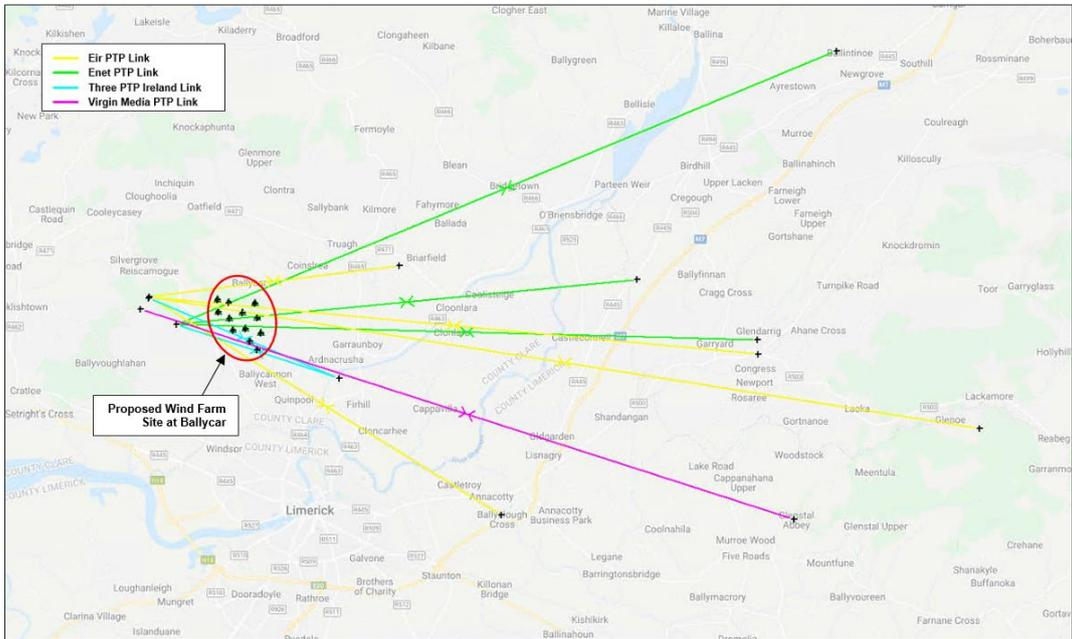
**Figure 1. Telecom Operator Networks shown relative to proposed wind farm site**
