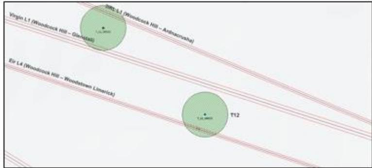
Figure 23. Close-up Plan View of T12 relative to nearest radio links
