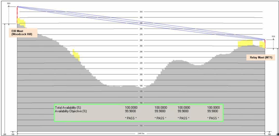
Figure 22. Woodcock Hill – Relay Mast Path Profile
