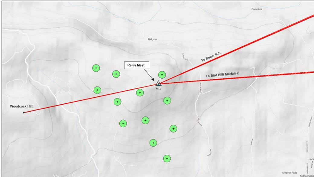
**Figure 9. Proposed Relay Mast Location and relay links to Boher N.S and Birdhill**
