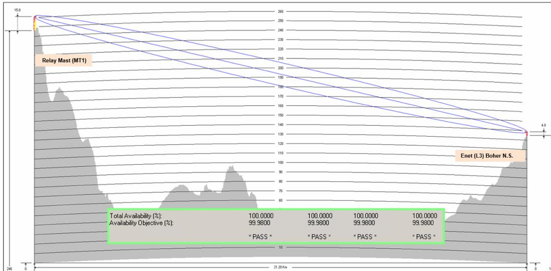
Figure 12. Relay Mast – Boher N.S. Path Profile
