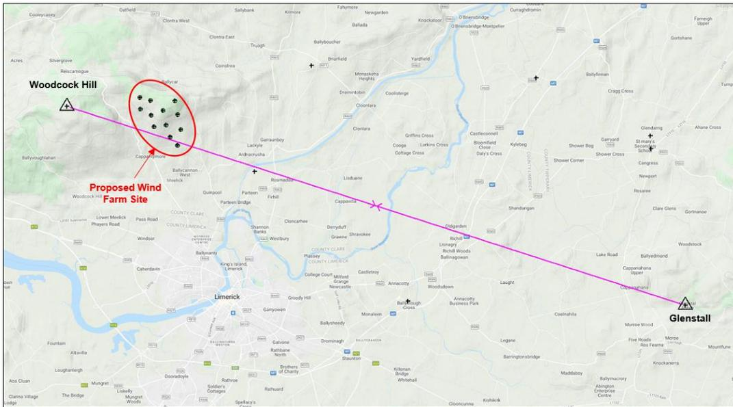
**Figure 35. Virgin Media Radio Network – Plan View**
