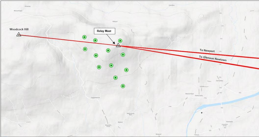
Figure 21. Proposed Relay Mast Location and relay links to Newport and Glenoue Newtown
