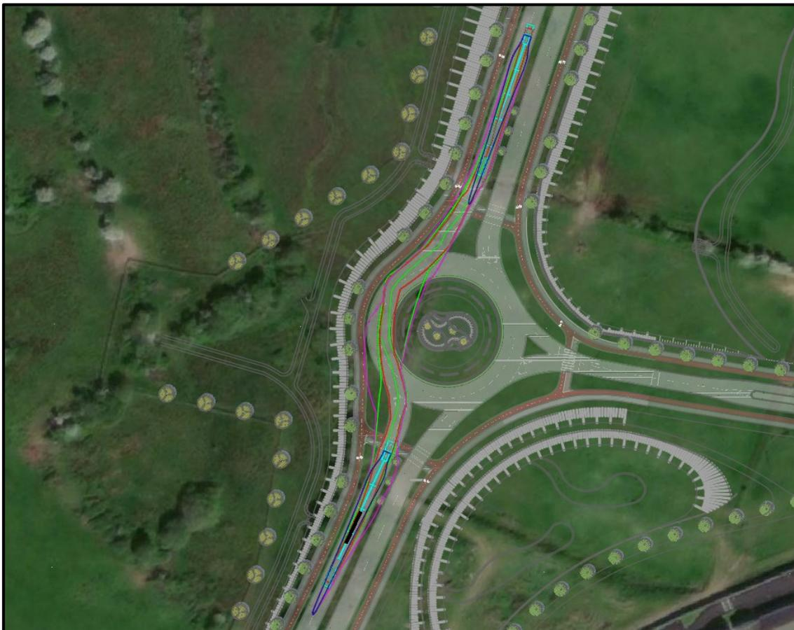
Figure 36: Moyross Roundabout – swept path
