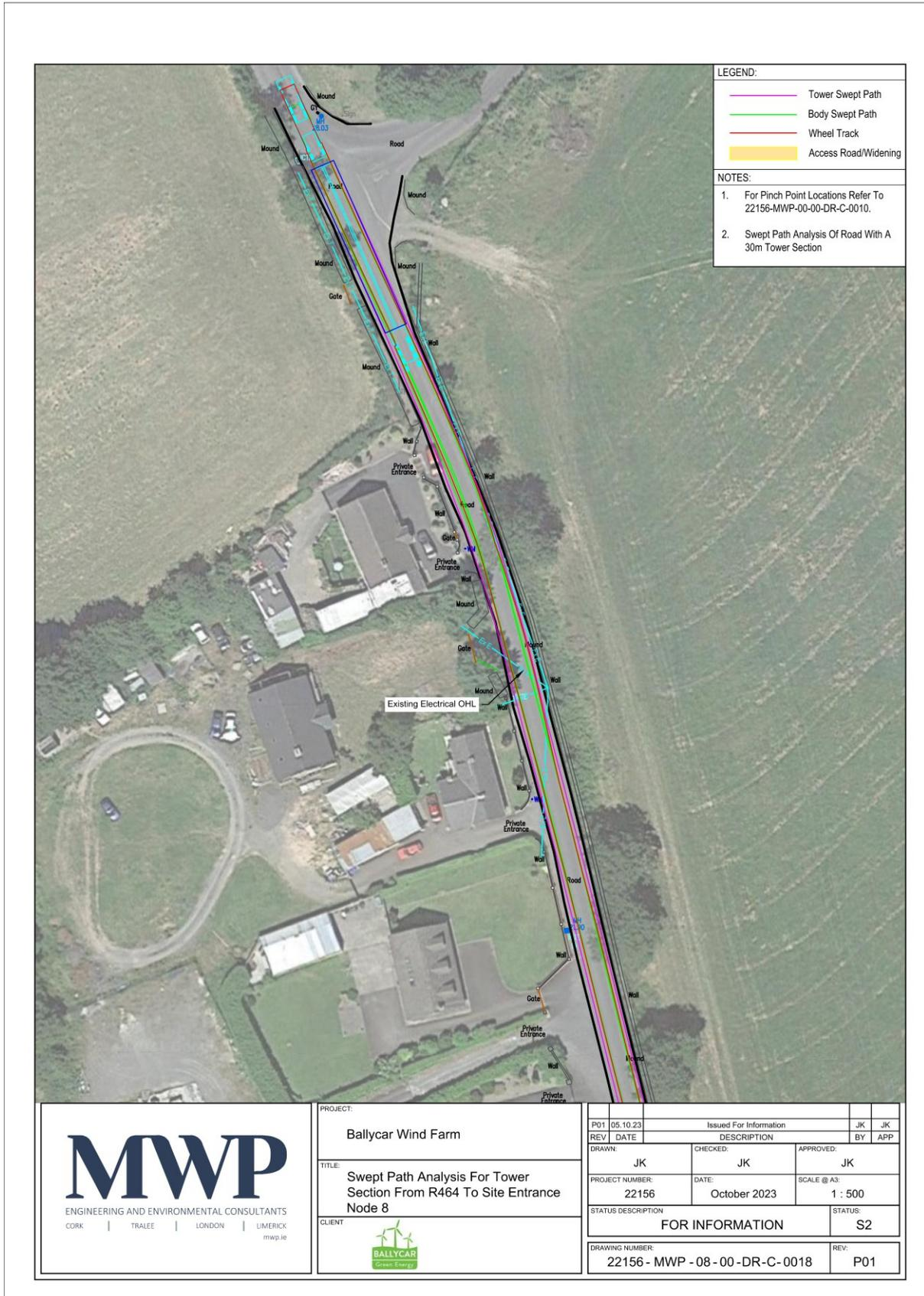
Figure 74: Area No. 8 –Tower section delivery – swept path
