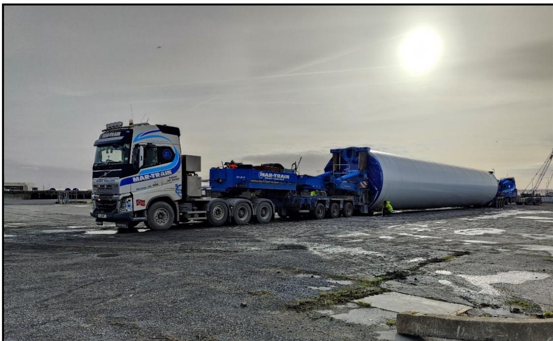
Figure 6: Bogie type tower transporter
