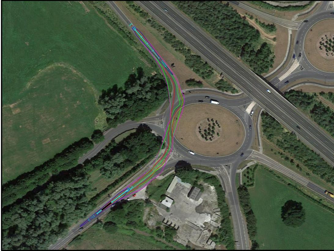
Figure 18: N69 Dock Road Roundabout to N18 on-ramp – swept path
