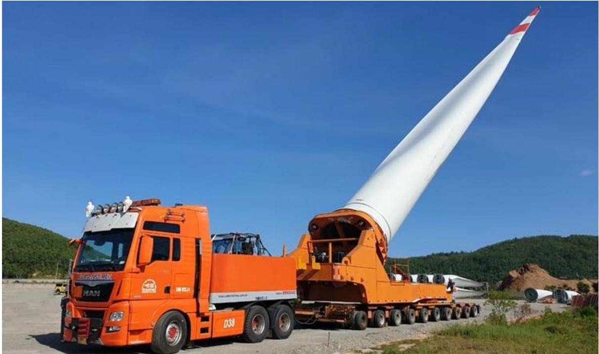
Figure 2: Blade lifter trailer with blade tilted to 60° to the horizontal
