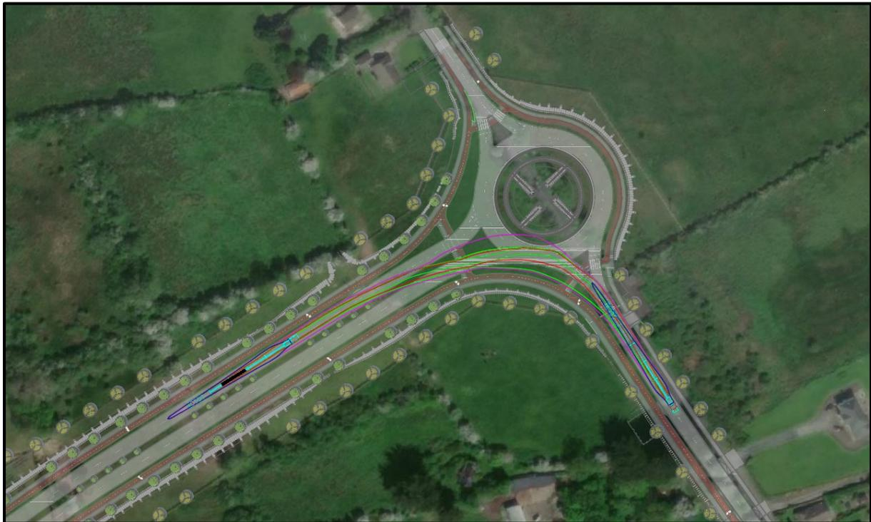
Figure 37: Knocknalisheen Road Roundabout – swept path
