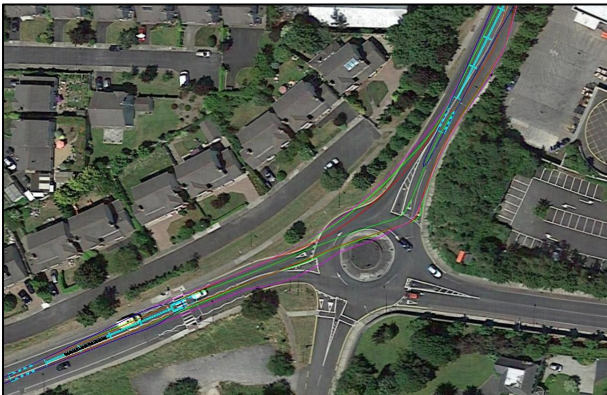
Figure 44: Roundabout on Clonmacken Road – swept path
