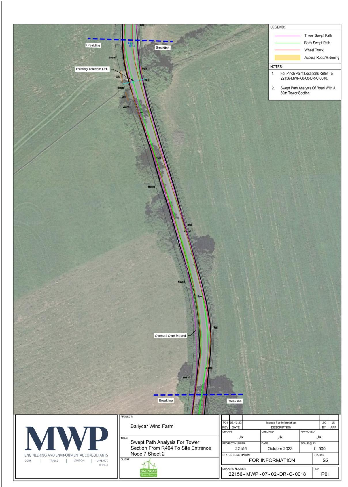
Figure 70: Area No. 7.2 – Tower section delivery – swept path
