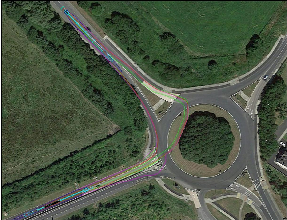
Figure 29: Clonmacken Roundabout – swept path
