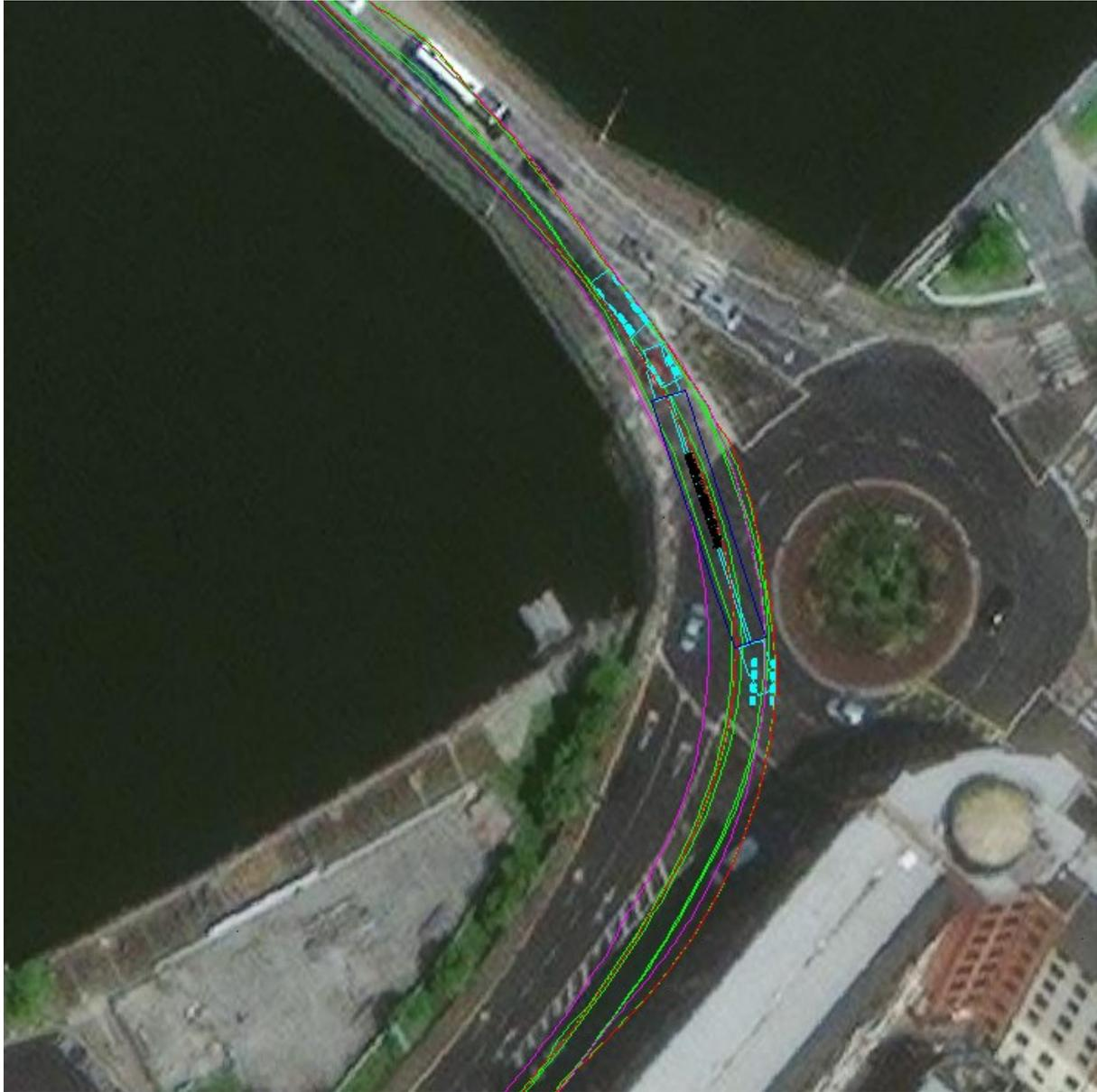
Figure 27: Shannon Bridge Roundabout and Condell Road R527 – Tower section swept path
