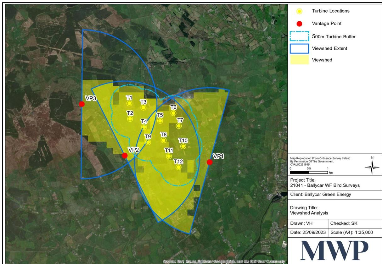
**Figure 3-3: The 500-metre buffer zone around the turbines, three Vantage Point (VP) locations, and the viewsheeds coverage of each VP.**
