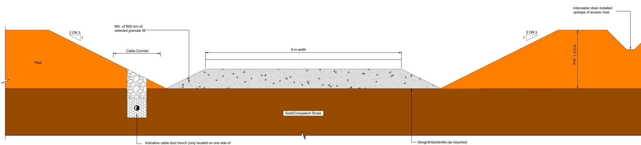
Indicative cable duct trench (only located on one side of the roadway across majority of the site). Cable trench can be located on either side of the road surface or below the road surface but where possible it should be located on the upslope side of the road surface.
