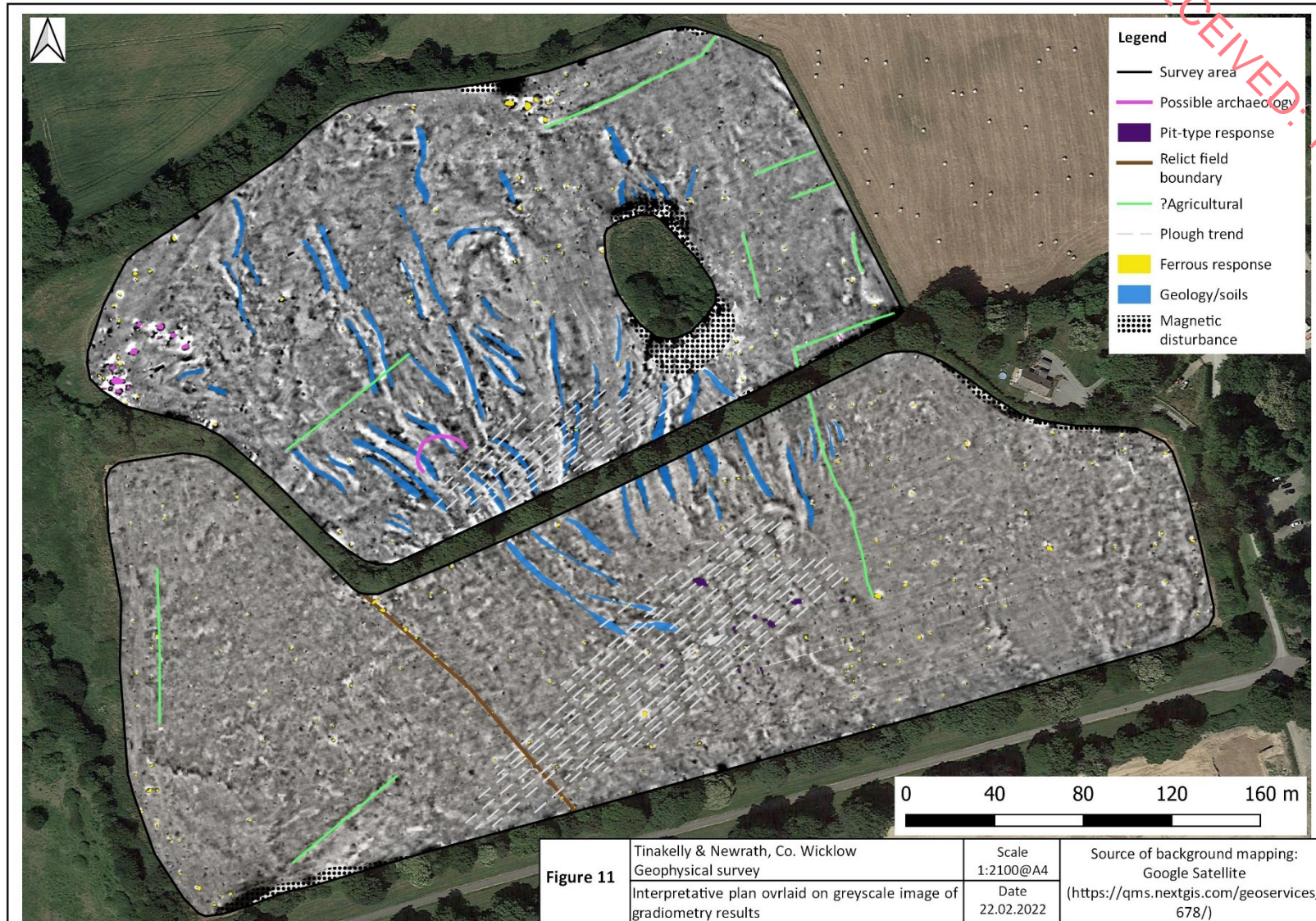
Figure 11. Interpretative plan overlaid on greyscale image of the gradiometry results.
