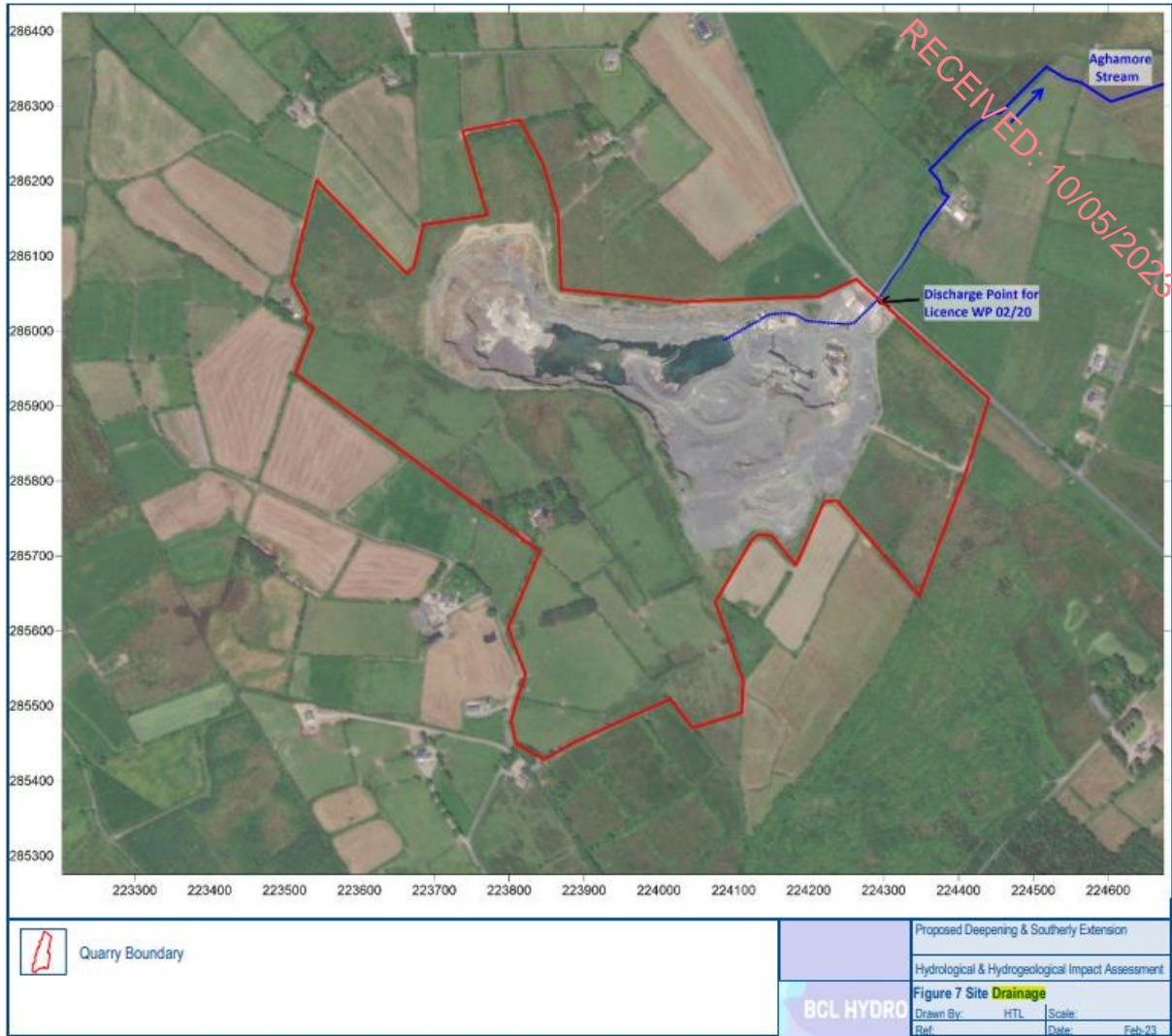
Figure 3: Site drainage as per the Hydrogeology and Hydrology Report (Source: BCL Hydro, 2023)
