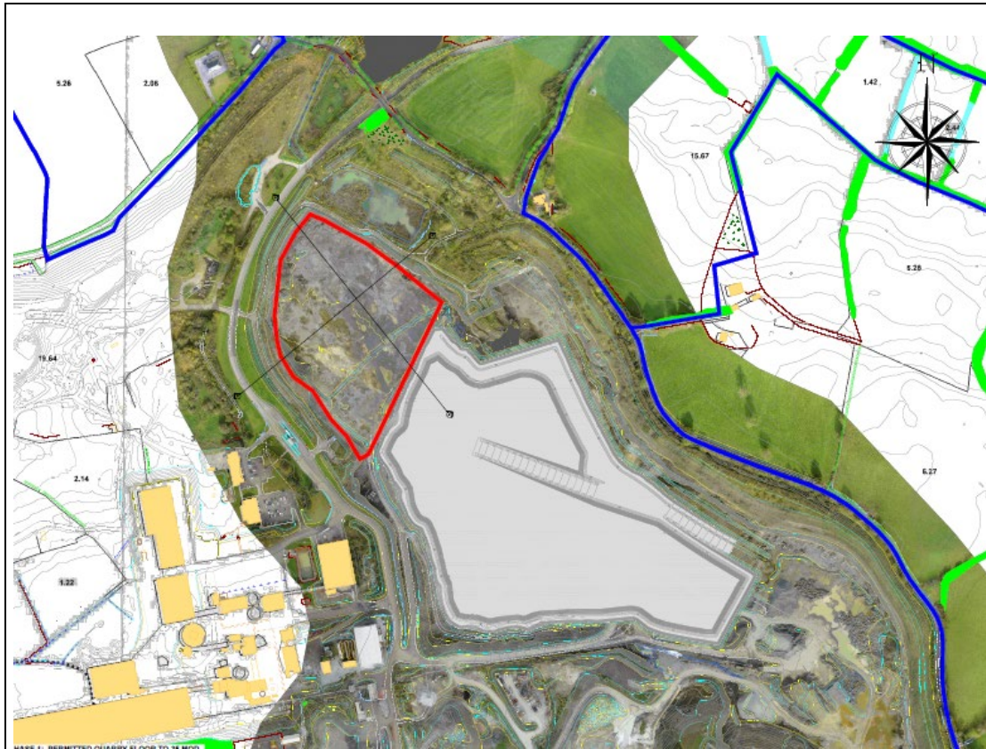
Figure 3.1 - Phase 1 of quarry extraction – adjacent areas extracted to 35m OD
