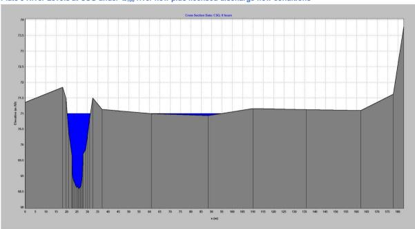
Plate 5 River Levels at CSG under  $Q_{100}$  river flow plus licensed discharge flow conditions
