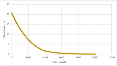
The Cooper-Jacob method is suitable for interpretation of pumping test and recovery test data providing certain assumptions are met. In this case the pumping phase did not achieve steady-state drawdown conditions.
