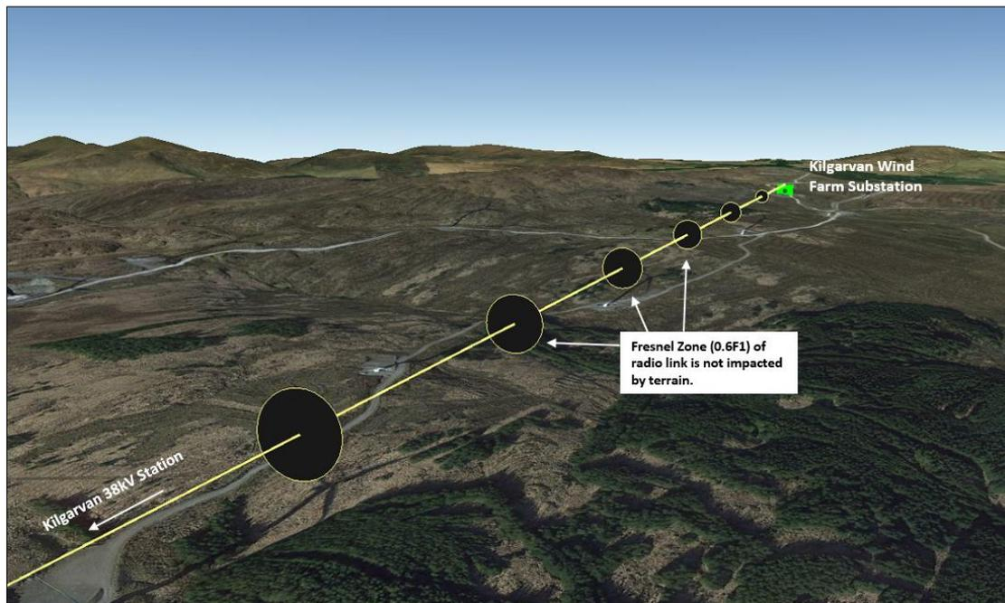
**Figure 9. 3D Model showing the Fresnel Zone (0.6F1) of the link is not impacted by terrain - ESB Link 1.**
