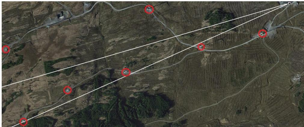
Our engineers completed a detailed analysis in relation to the proposed Re-powering project of Kilgarvan Wind Farm development. Our engineers incorporated the correct co-ordinates in their analysis which shows that there may be an impact from only one of the proposed wind turbines on the 0.6F1 Fresnel Zone. Please note that our engineers have used this reference as the basis of 0.6F1 Fresnel Zone analysis
