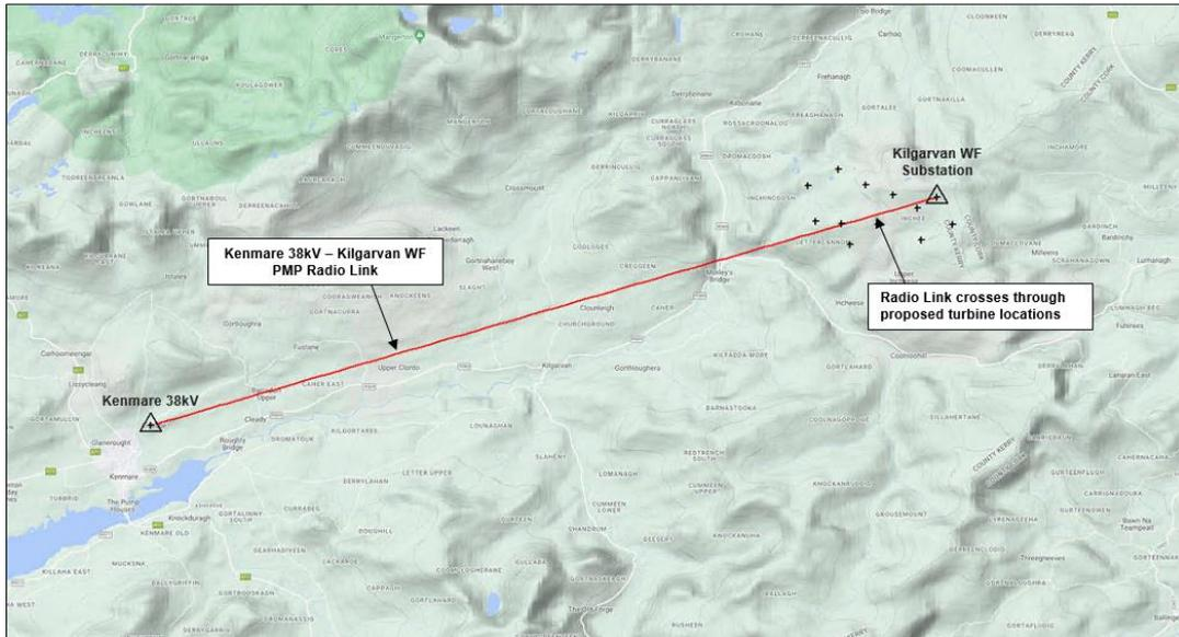
**Figure 11. ESB’s radio link between Kilgarvan 38 kV and Kilgarvan WF Substation.**
