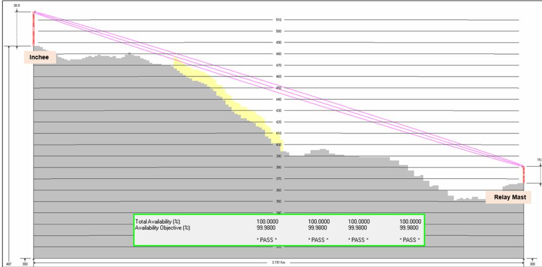
**Figure 25. Path Profile – Inchee to Proposed Relay Mast**
