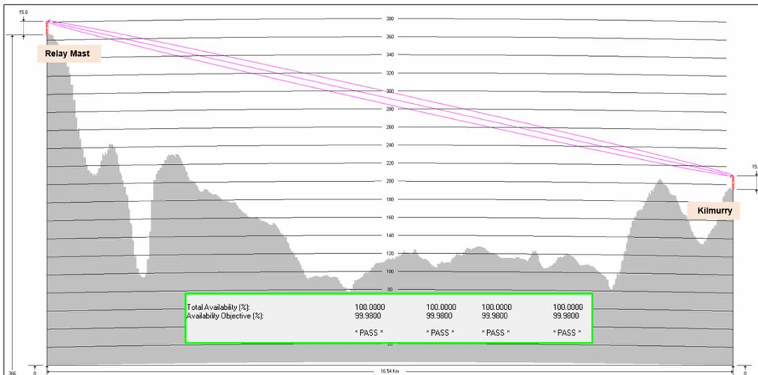
**Figure 26. Path Profile – Proposed Relay Mast to Kilmurry**
