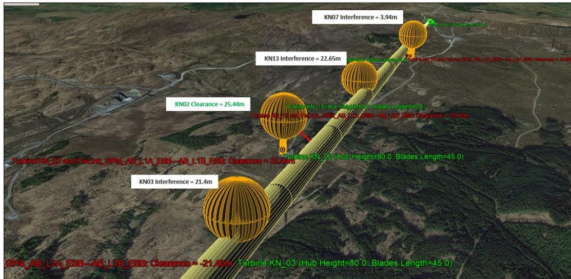
**Figure 10. 3D Model showing that the radio link path is obstructed by existing turbines - ESB Link 1.**
