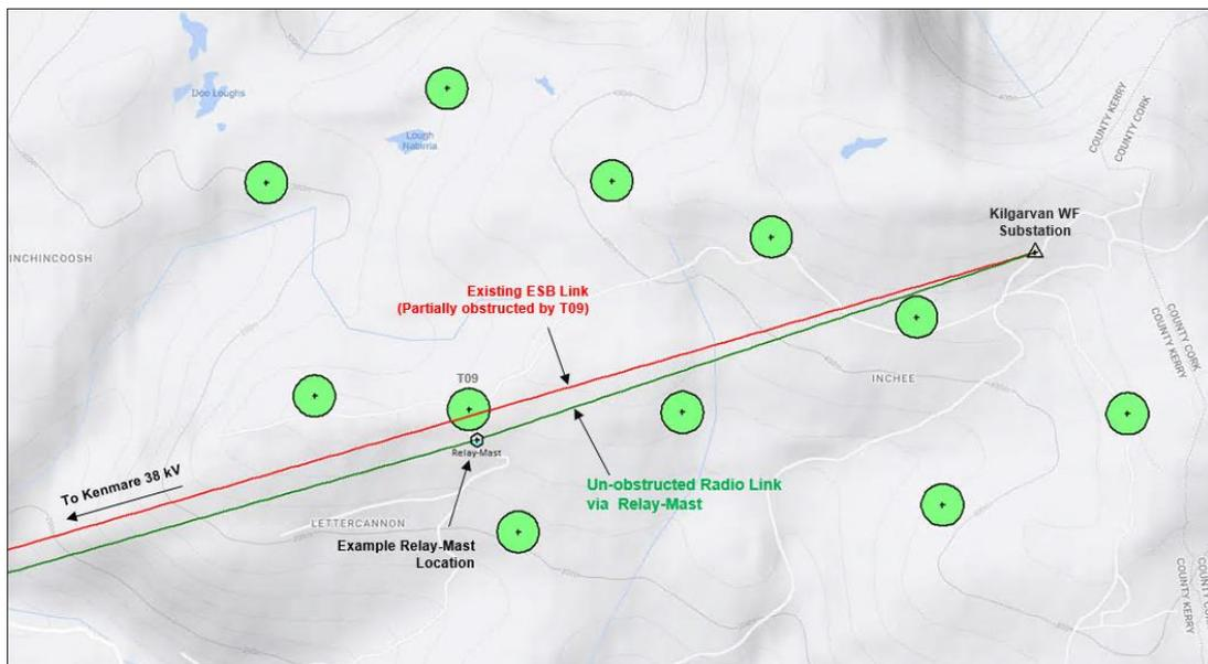
**Figure 14. Example of a relay mast used to mitigate against an obstructing turbine.**
