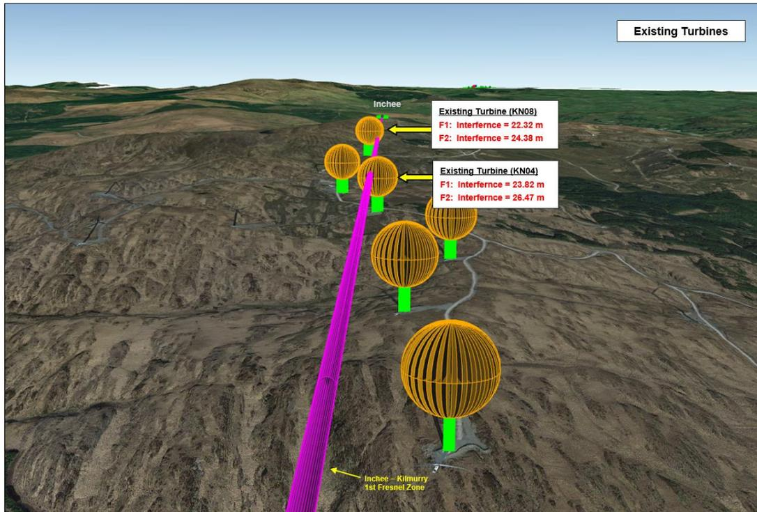
Figure 14. 3D Model showing that the Fresnel Zone of the radio link is obstructed by two existing turbines.
