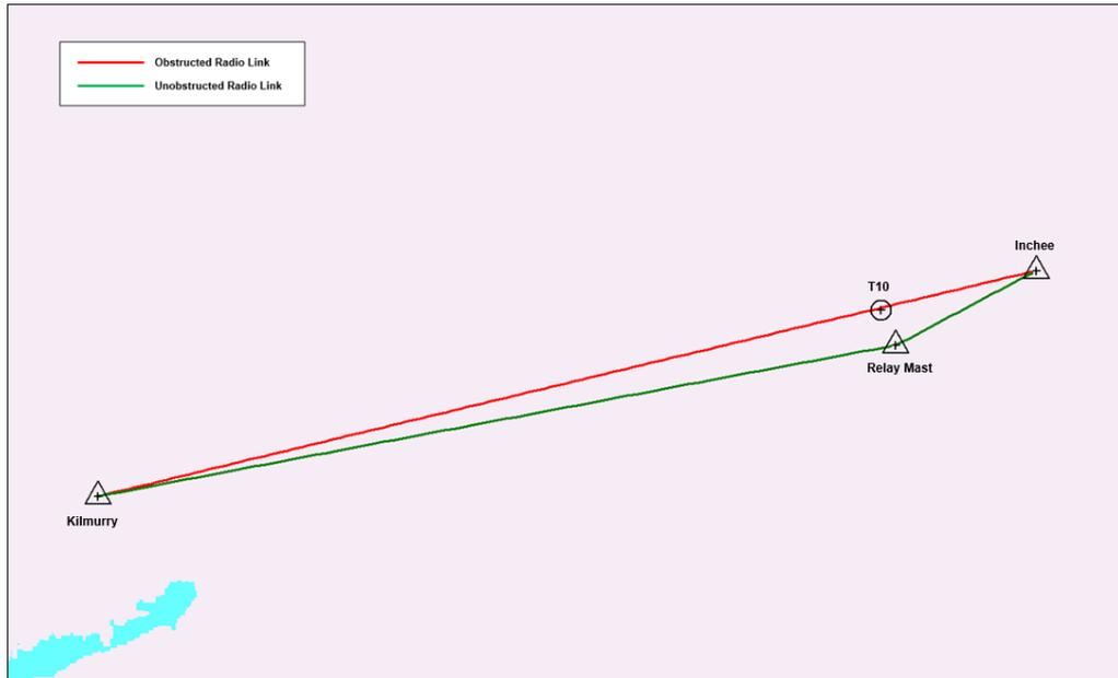
**Figure 22. Illustration of how a relay mast could be used to mitigate against an obstructing turbine.**
