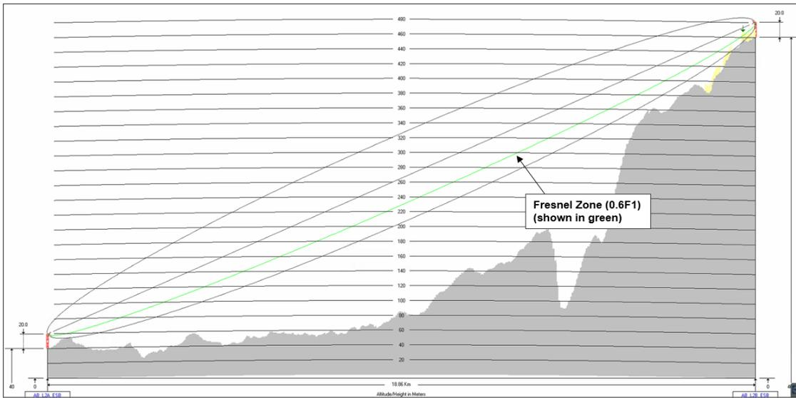
**Figure B.2 ESB Link 2 Path Profiles (Kenmare 38kV – Kilgarvan Wind Farm Substation)**
