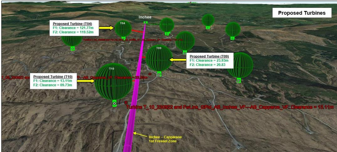
Figure 10. 3D Model showing proposed Re-Powering turbines relative to the Vodafone Radio Link.
