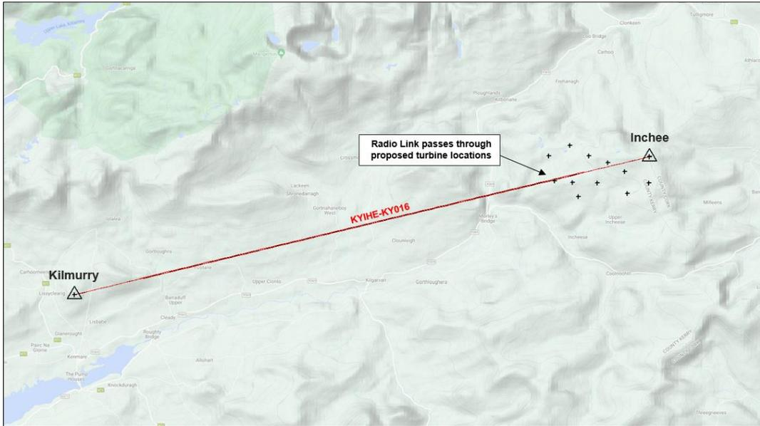
**Figure 12. Vodafone’s radio link between Inchee and Kilmurry.**
