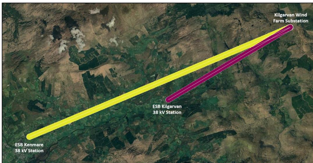
Figure 2. Plan View of ESB PMP Radio Links
