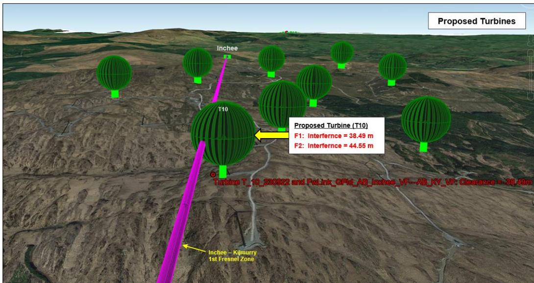
**Figure 13. 3D Model showing proposed Re-Powering turbines relative to the Vodafone Radio Link.**
