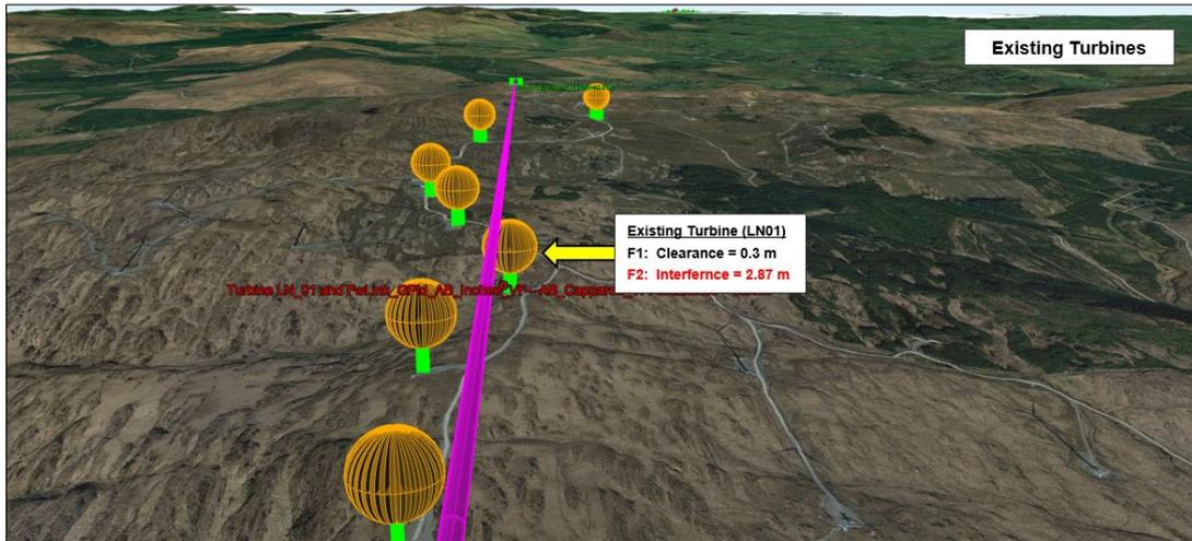
Figure 11. 3D Model showing that that 2<sup>nd</sup> Fresnel Zone of the radio link is partially obstructed by an existing turbine.
