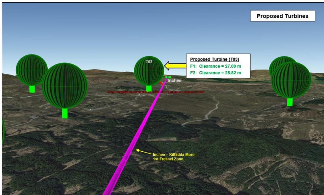
**Figure 16. 3D Model showing proposed turbines relative to the Vodafone Radio Link.**
