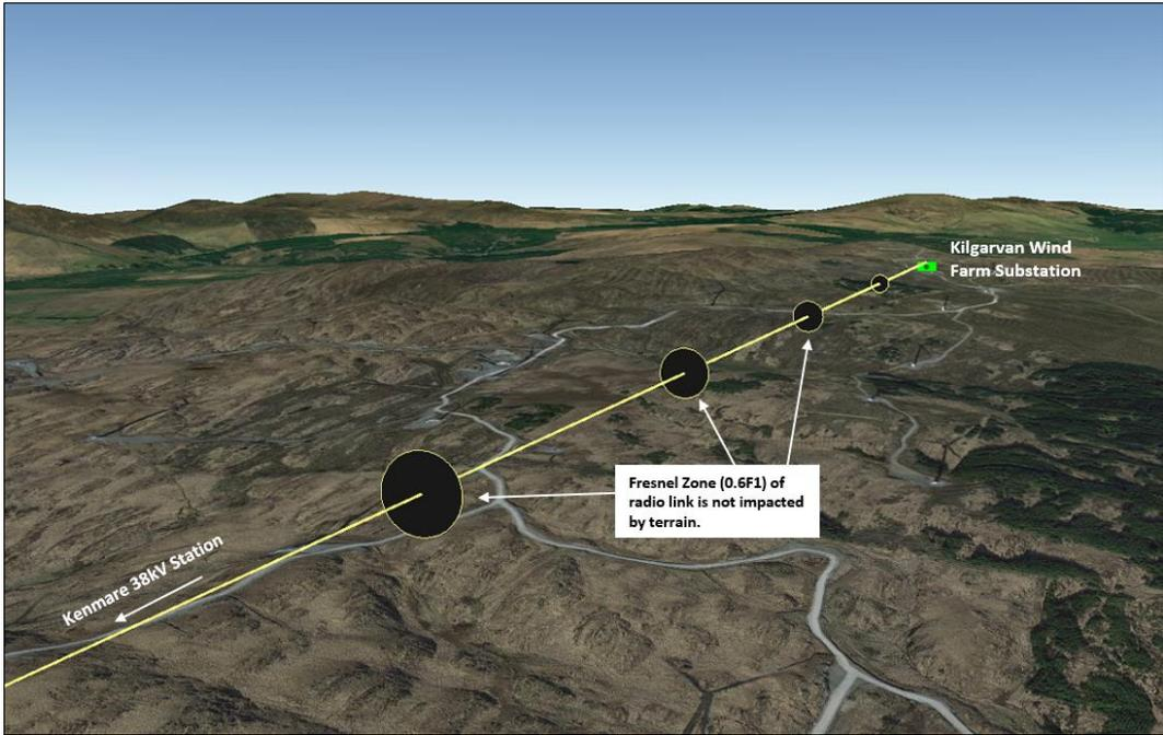
Figure 13. 3D Model showing the Fresnel Zone (0.6F1) of the link is not impacted by terrain - ESB Link 2.
