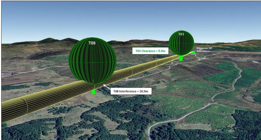
**Figure 8. 3D Model showing proposed Re-Powering turbines relative to the radio link – ESB Link 1.**
