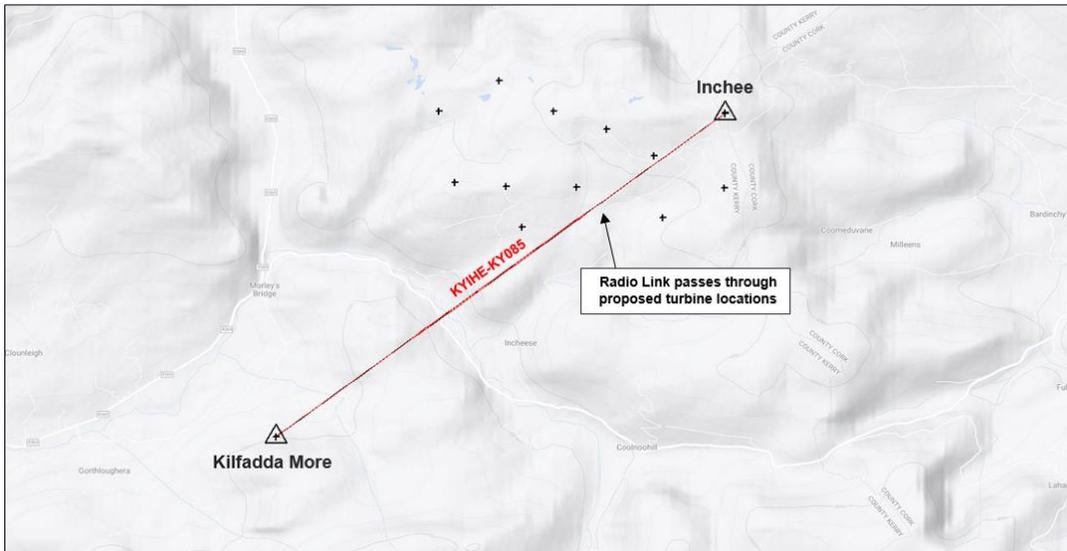
**Figure 15. Vodafone’s radio link between Inchee and Kilmurry.**
