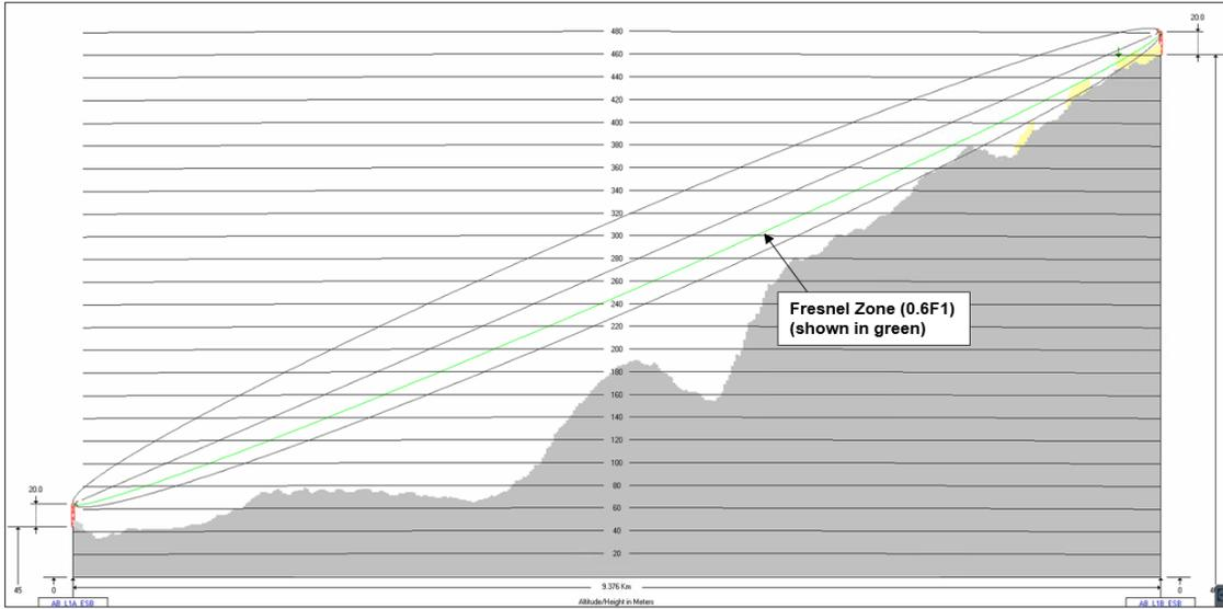
**Figure B.1 ESB Link 1 Path Profile (Kilgarvan 38kV – Kilgarvan Wind Farm Substation)**
