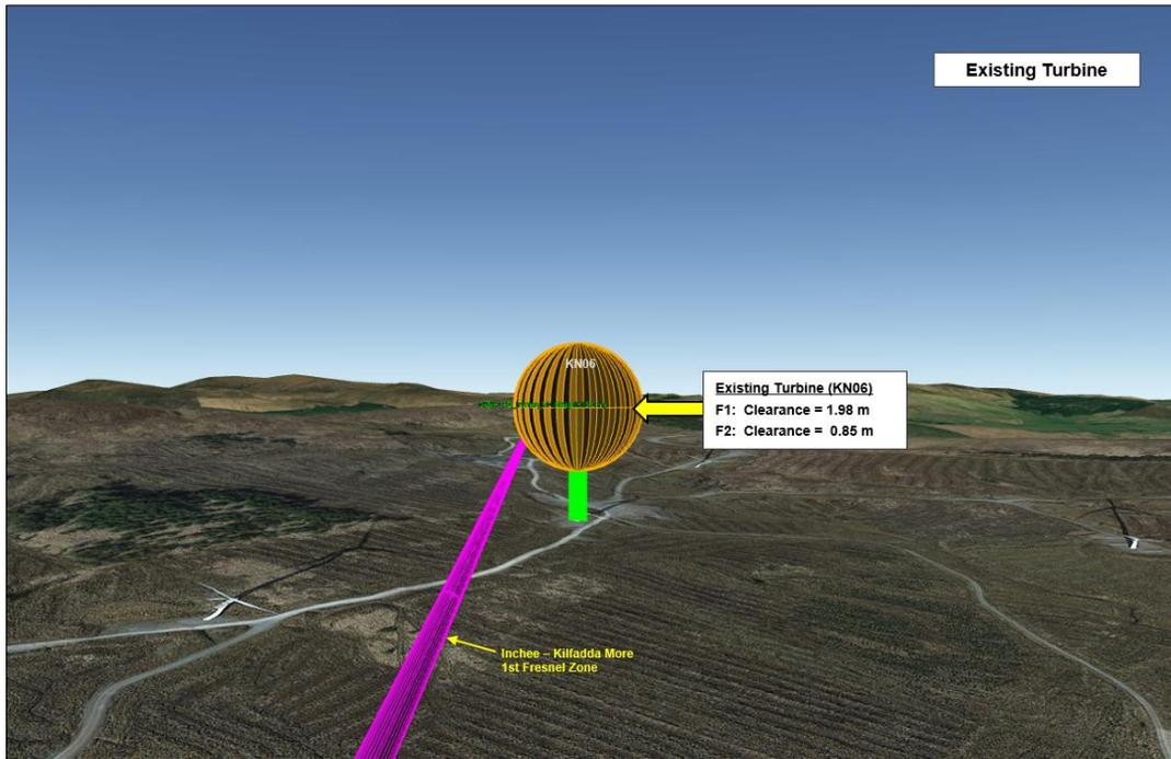
Figure 17. 3D Model showing existing turbine which is less than 2m from the radio link Fresnel Zone.
