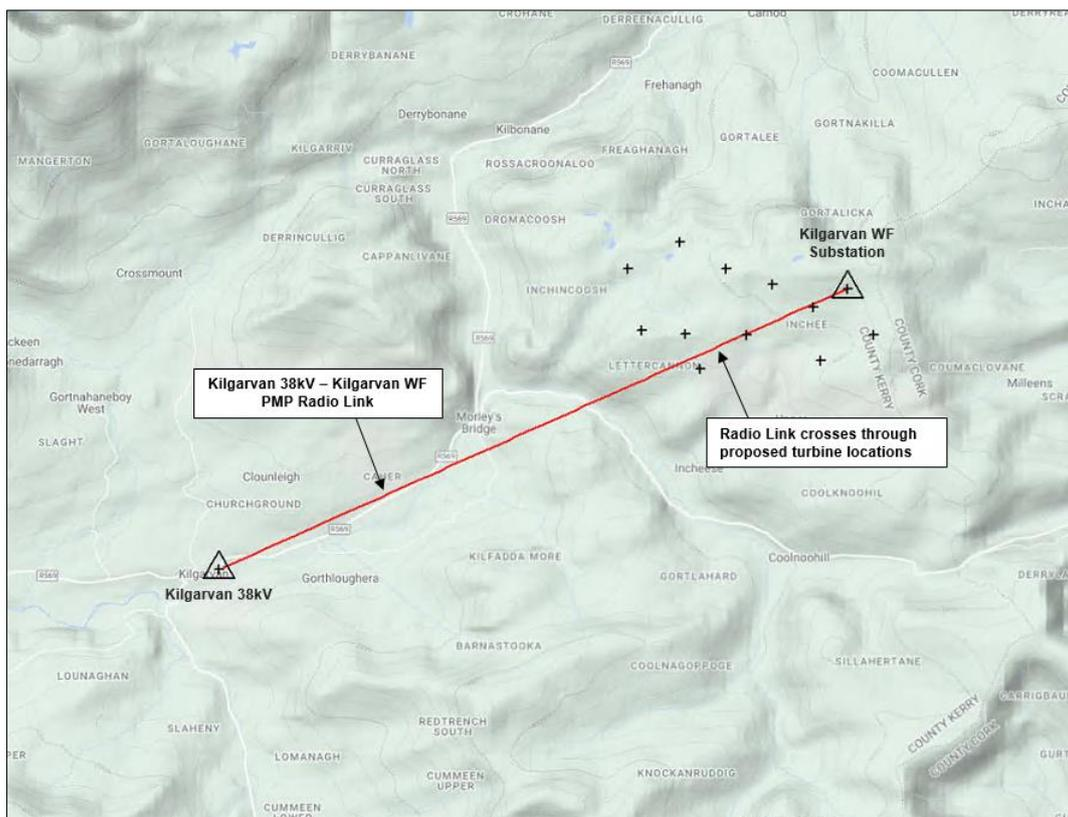
**Figure 7. ESB's radio link between Kilgarvan 38 kV and Kilgarvan WF Substation.**
