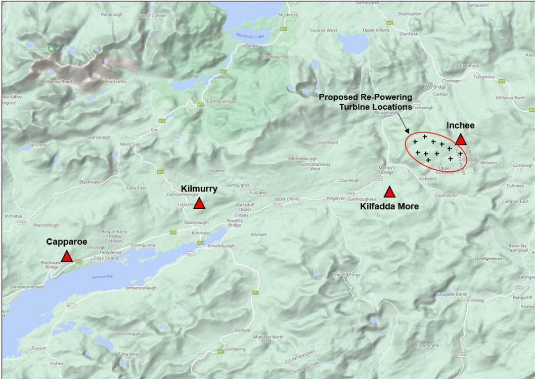
**Figure 4. Location of the Proposed Development relative to Vodafone Radio Link mast-sites**
