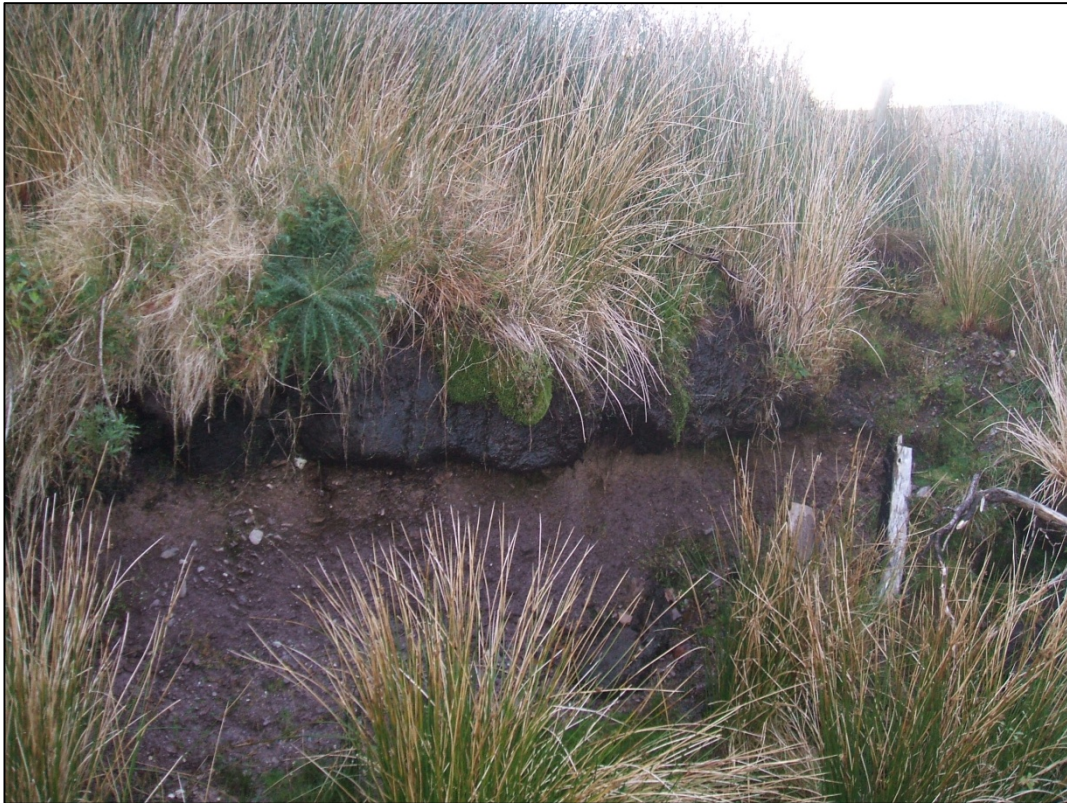
Photo 5 Example of creep movement of peat on site
