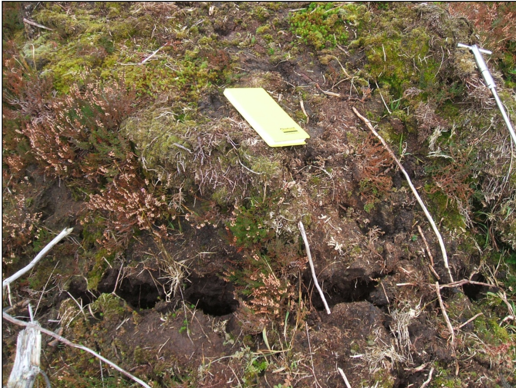
Photo 3 Tension cracks in the peat surface about 10m behind the failure scar
