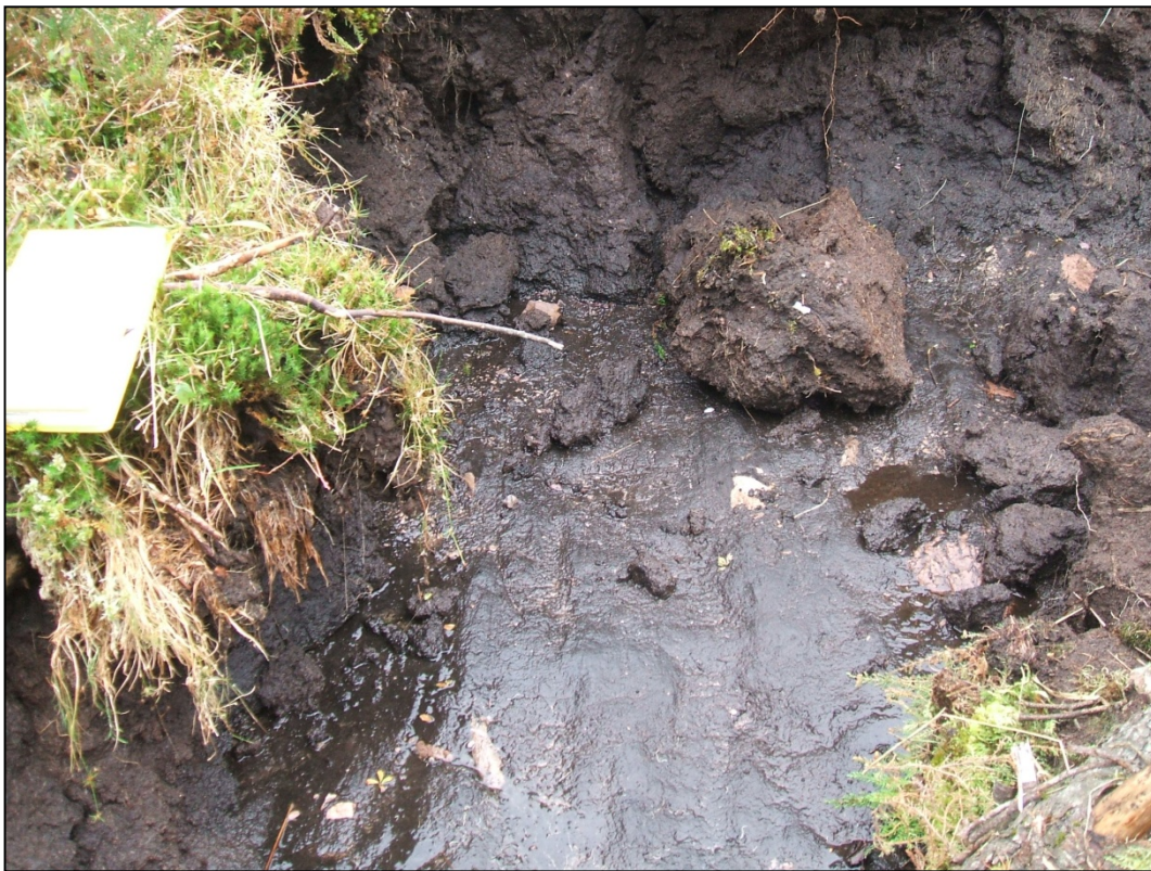
Photo 4 Basal shear surface of the failure
