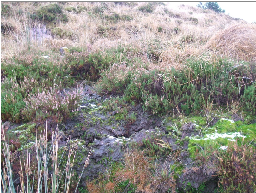
Photo 10 Localised relict tension cracks south of turbine T17
