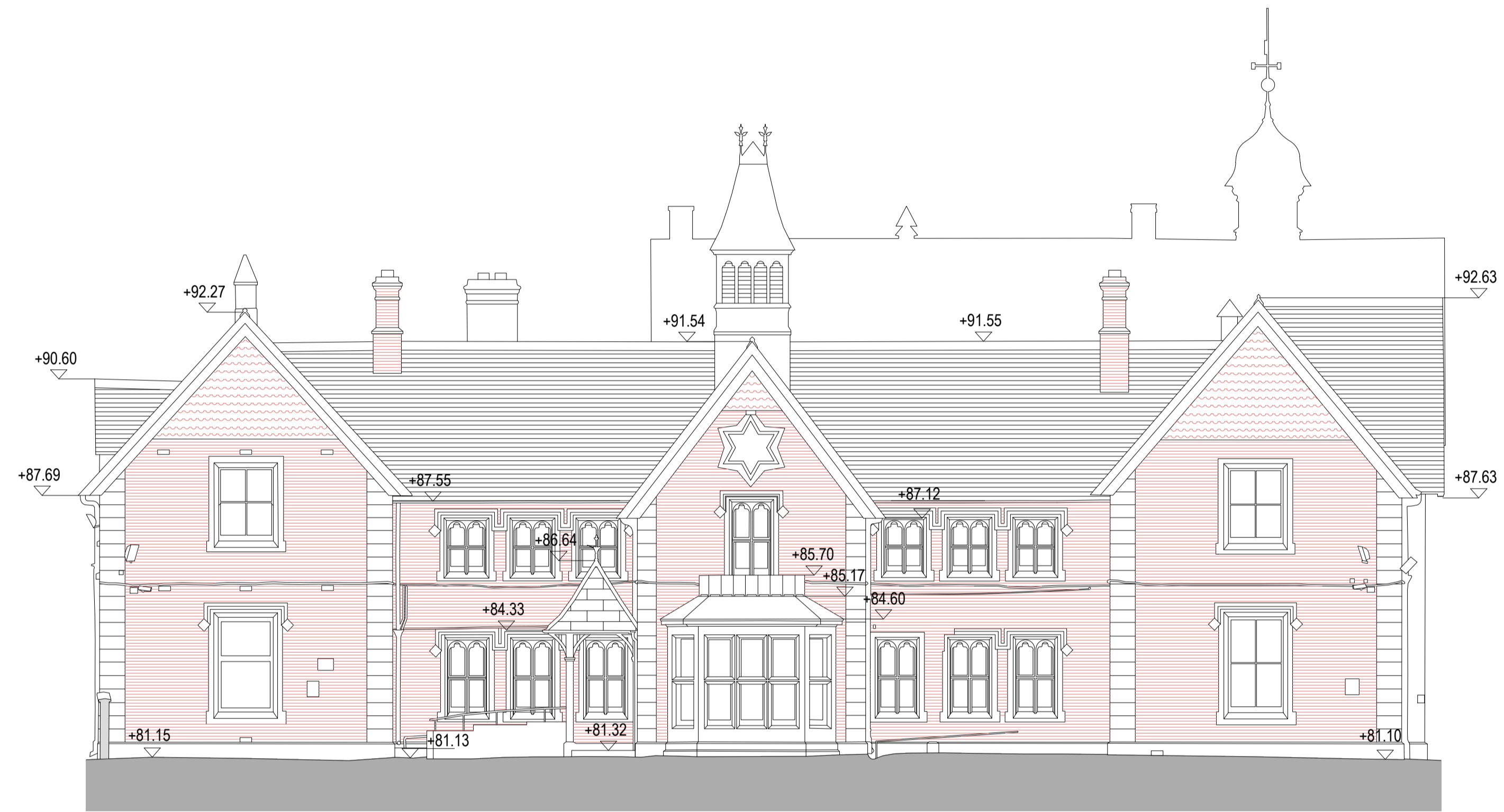
SURVEY ELEVATION 03 - NORTH EAST SCALE 1:100
