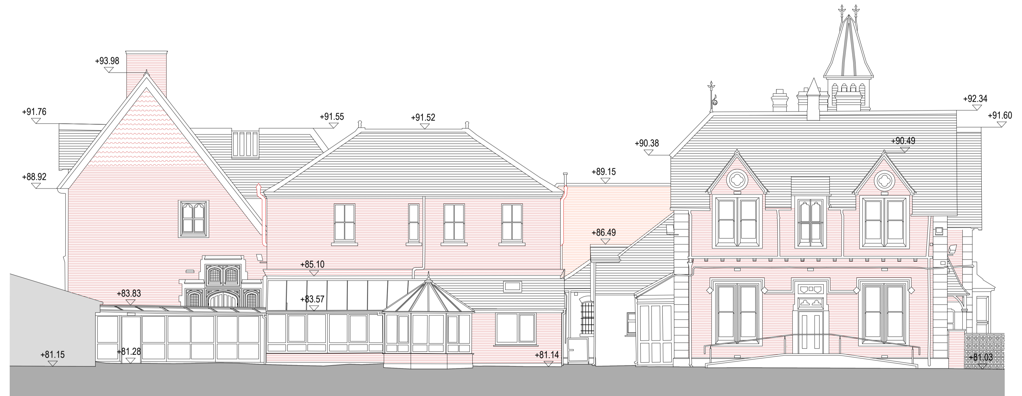
SURVEY ELEVATION 02 - SOUTH EAST SCALE 1:100
