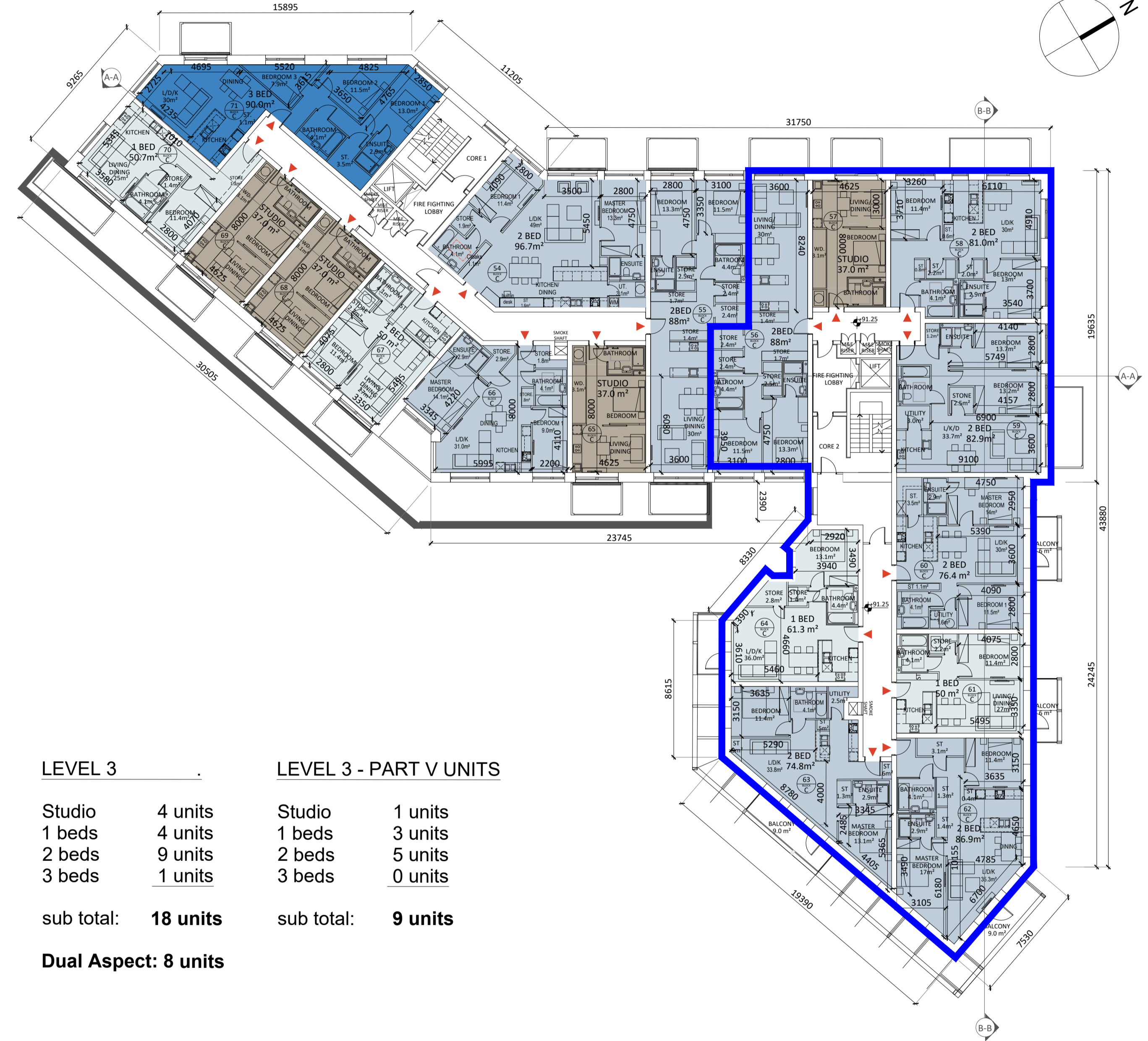
THIRD FLOOR LEVEL - BLOCK C SCALE 1:200
