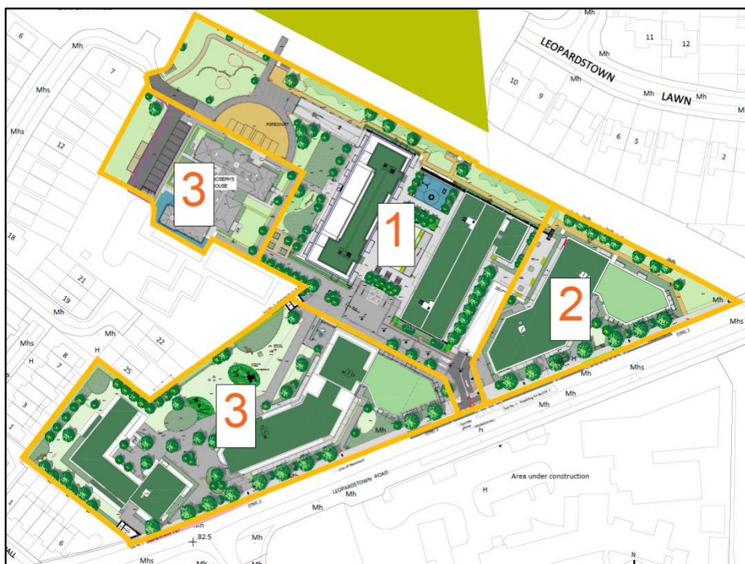
Figure 3.4 - Site Construction Phasing Strategy
