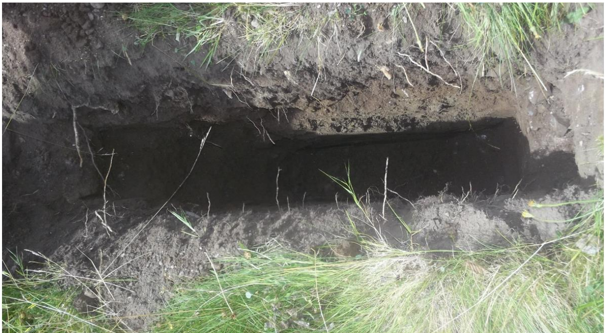
Test Pit before water added – Depth 1.2m
