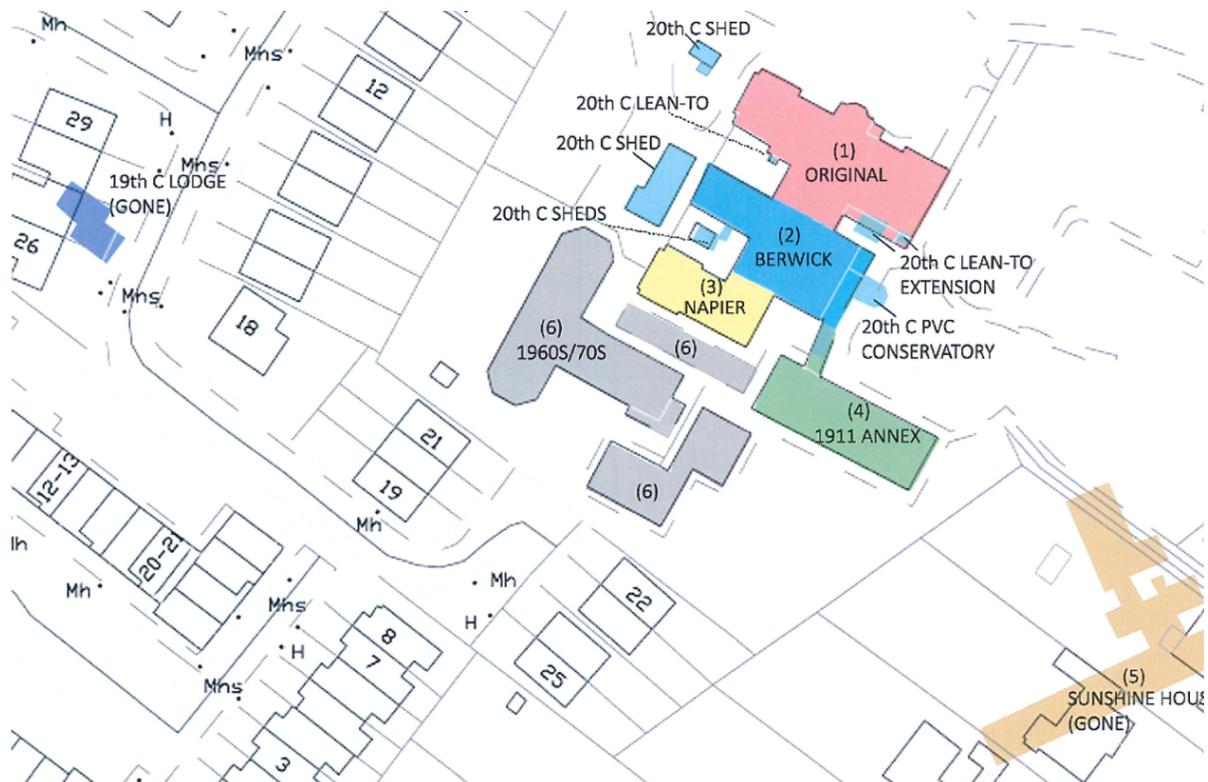
Figure 5: Fabric chronology plan showing the phases of development of the former Convalescent Home, overlaid on the current Ordnance Survey. The original footprint and the Napier and Berwick phases of development which quickly followed are clearly visible here. Also visible are the footprints of the 20th Century sheds, lean-to extensions, annex and conservatory. The footprint of the gate lodge to the original western entrance is also visible here within Silver Pines.
