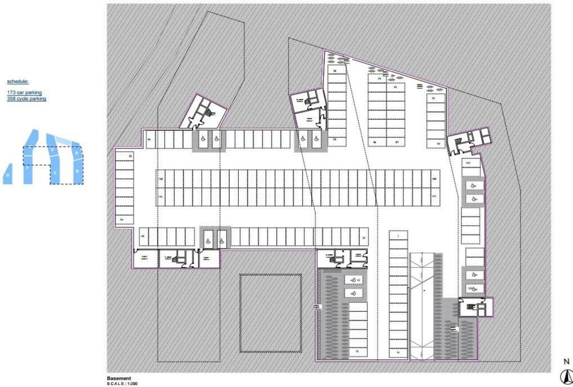
Fig. 14.4 Plan of the basement layout for the proposed development
