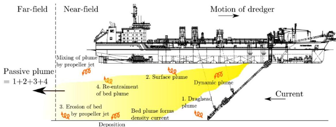
Plate 6-37 Mechanisms for release of sediment from TSHD dredging. Figure reproduced from Becker et al. (2015).
