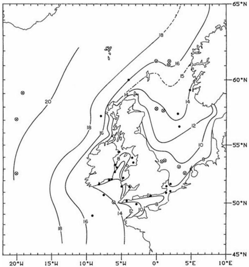
Plate 6-4 Isopleth contour map of indicative values of 50-year return period significant wave height (m). Figure reproduced from Carter (1993)
