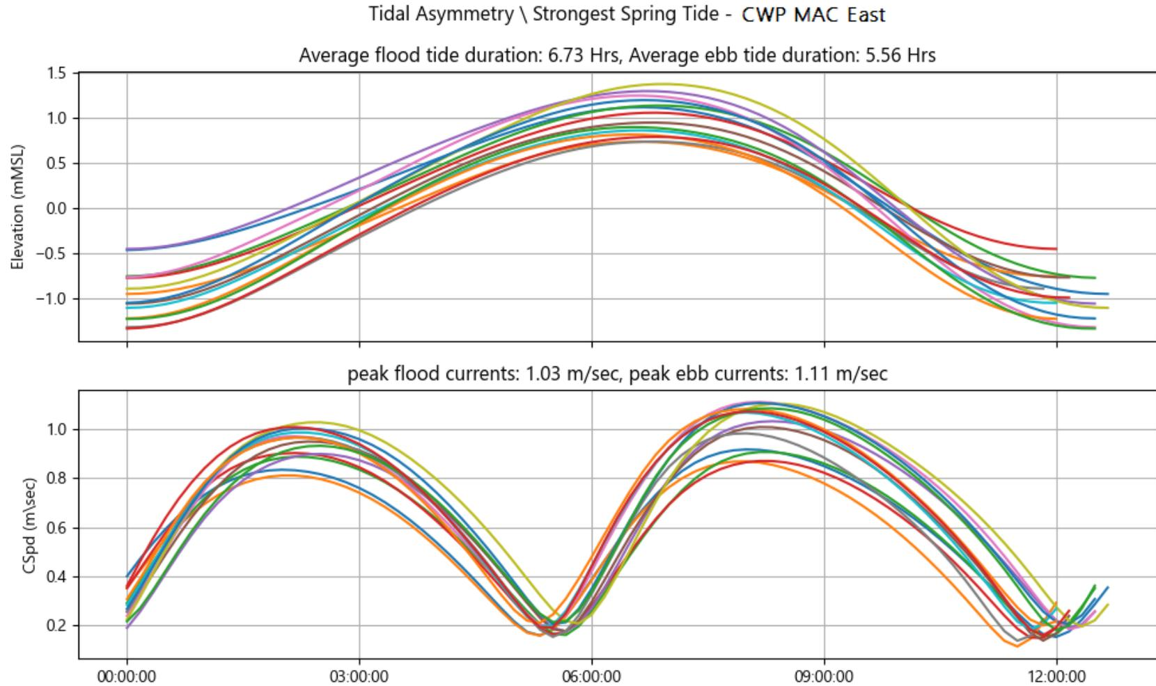
Plate 6-11 The predicted ebb dominance at model point CWP MAC East during a typical spring tide. Water elevations (above) and current speeds (below) are shown.
