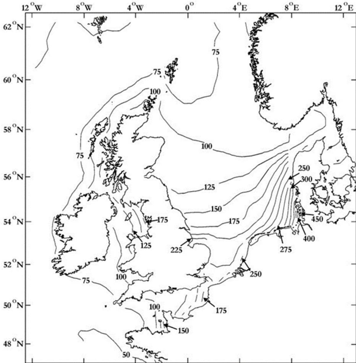
Plate 6-2 Isopleth contour map of 50-year return period storm surge elevations in cm (figure reproduced from Flather, 1987)
