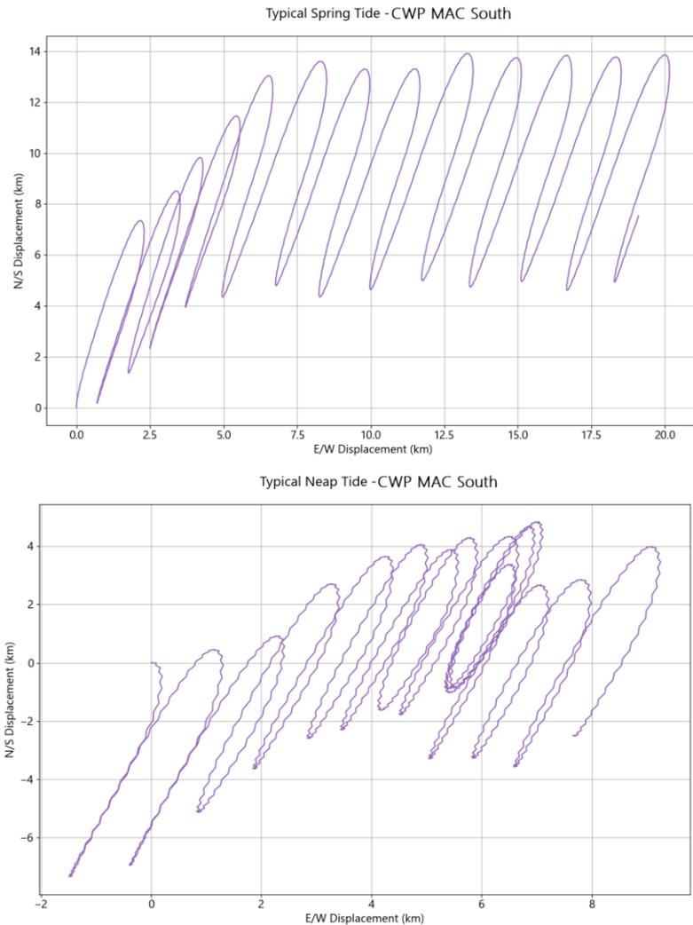
Plate 6-10 Illustrative tidal excursion (progressive vector) plot for model point CWP MAC South during the spring tidal phase (top panel) and the neap tidal phase (bottom panel)
