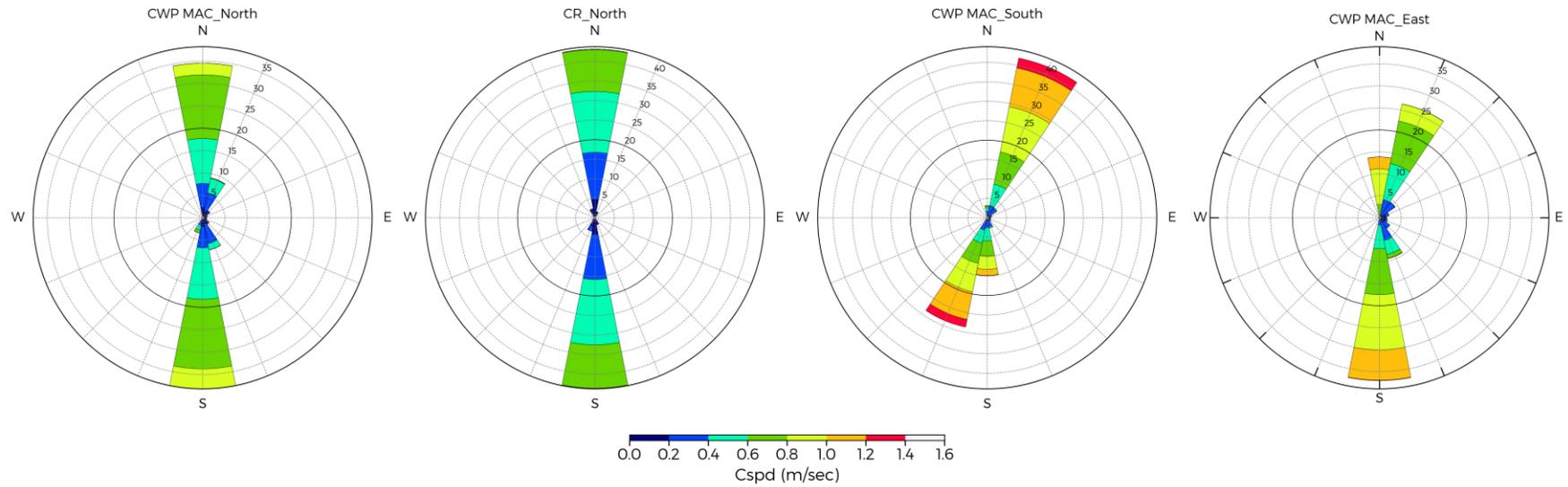
Plate 6-7 Current rose plots showing depth-averaged current speeds as a function of direction. Data presented are taken from the four model extraction points.
