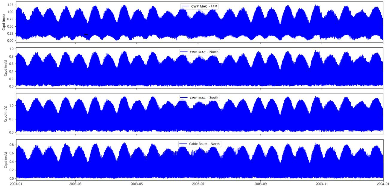
Plate 6-6 Depth-averaged current speeds predicted to occur at the four model extraction points plotted in the form of a timeseries. A representative period from the hindcast data record is presented (2003 to 2004).
