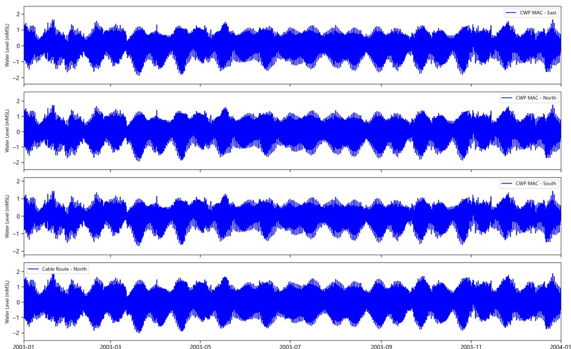
Plate 6-5 Water elevations predicted to occur at the four model extraction points plotted in the form of a timeseries. A representative period from the hindcast data record is presented (2003 to 2004)
