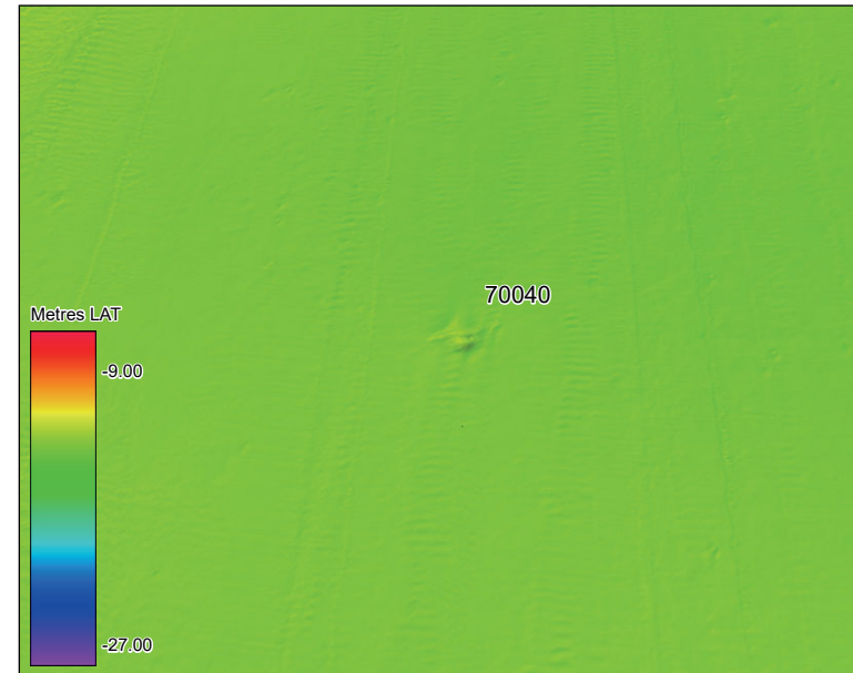
Gridded multibeam echosounder image showing debris field anomaly 70040 (Figure 7c), x1 vertical exaggeration
