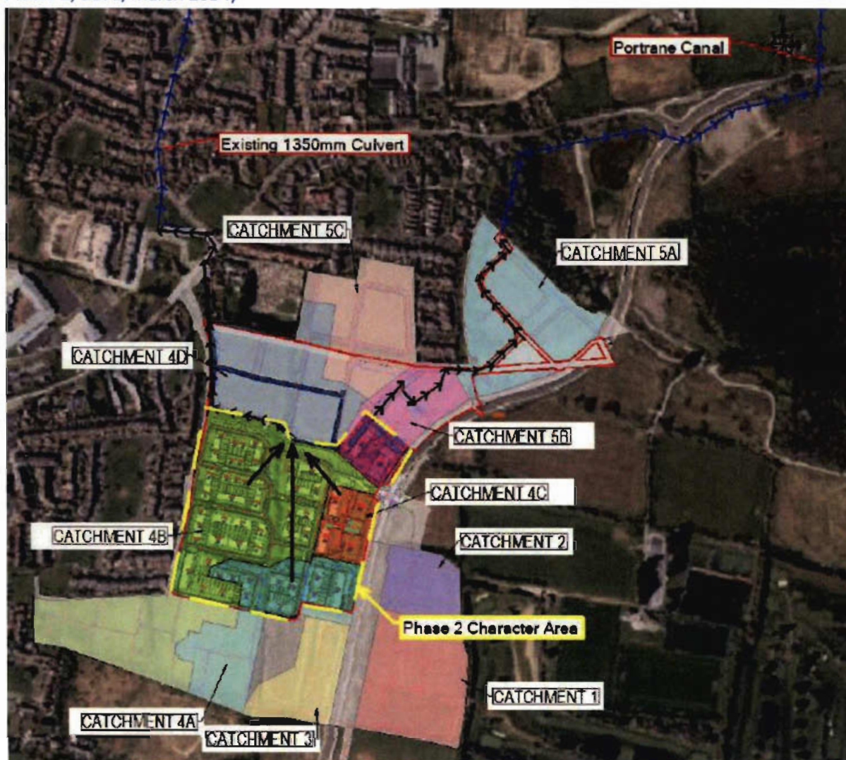
Figure 10.2 Masterplan Surface Water Catchment Plan (Source: Figure 6, Infrastructure Design Report Phase 2, DBFL, March 2024)
