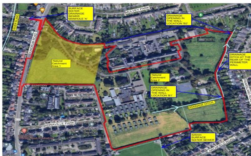
Fig 3.1. Aerial View of the Approximate Natural Catchment Areas and surface water drainage outfalls on the Existing Site. Catchment 1 shaded yellow. Catchment 2 is in the unshaded area.
