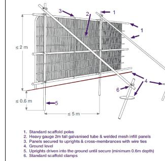
The tree protection fencing is to be erected enclosing the root protection areas around the trees being retained as shown on this drawing and appendix 1. In some areas, the site hoarding may be sufficient to act as the protective fencing if the tree and its root zone are positioned outside and no works are envisaged within the area outside the site hoarding. This will need to be discussed and agreed at the initial site meeting.
