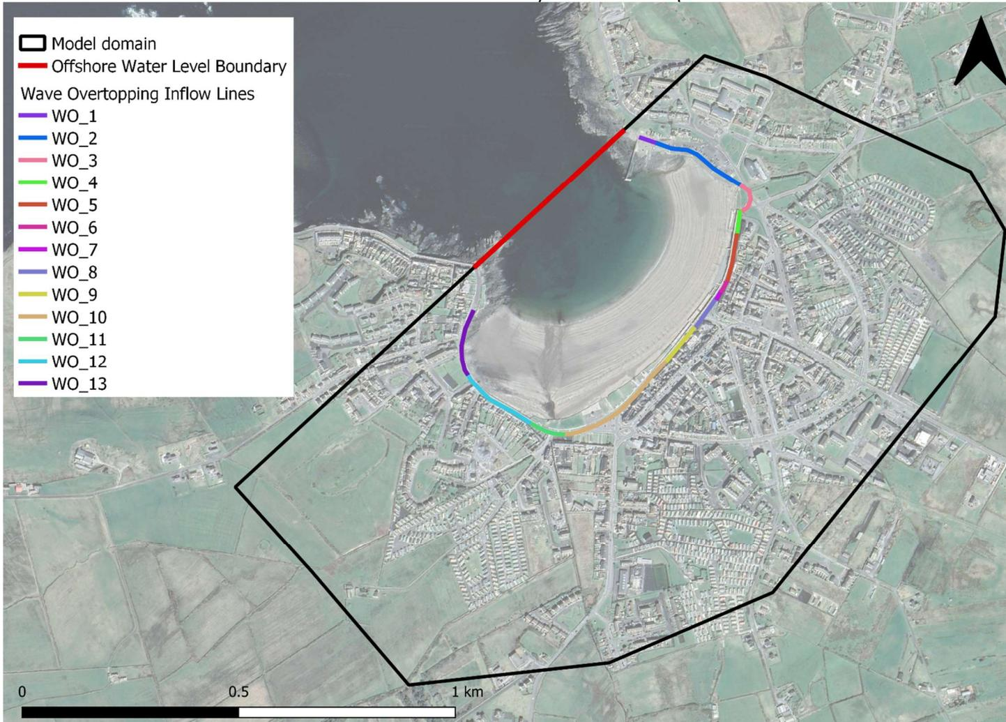
Figure 2-5. The model was constructed using a 2m resolution fixed grid suitable to pick out the key overland coastal flood flow paths.
