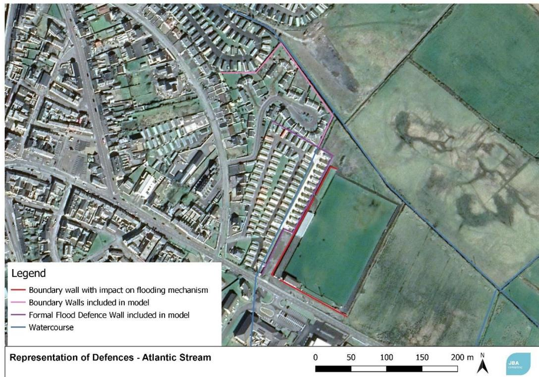
**Figure 3-9: Walls retained in Atlantic Stream Model**
