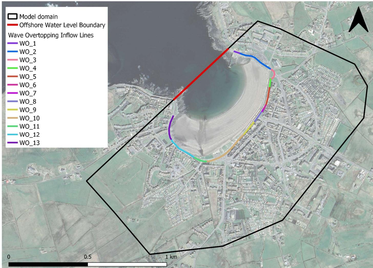
**Figure 2-5: Model domain and boundary location**
