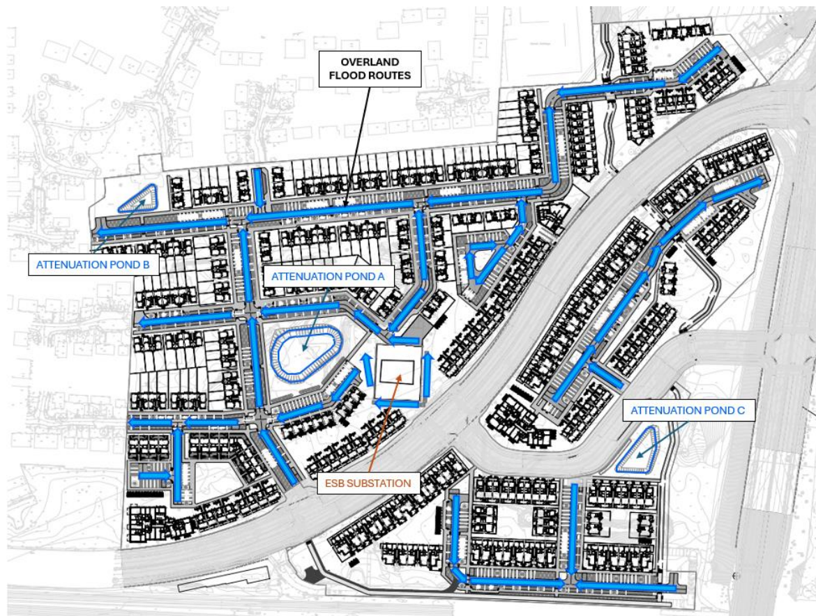
Figure 6.2 Proposed Overland Flood Routing
