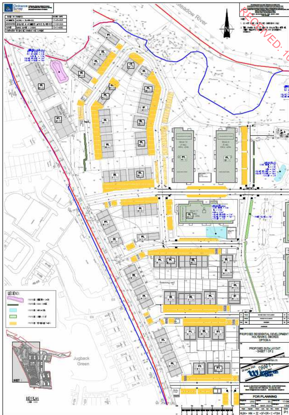
FIGURE 5. SUDS LAYOUT (WESTERN) (TOWNHOUSE) (DRG NO. P204, WATERMAN MOYLAN 2025).
