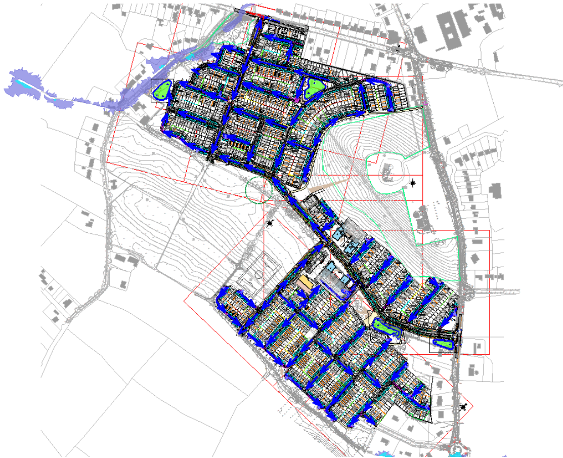
Figure 5-1 Flood Exceedance (>1% AEP) Overland Flow Paths
