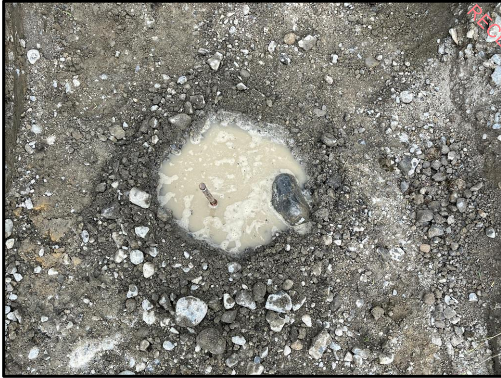
Figure 8: Shows subsurface and surface percolation test carried out.
