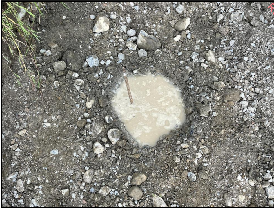
Figure 10: Shows subsurface and surface percolation test carried out.
