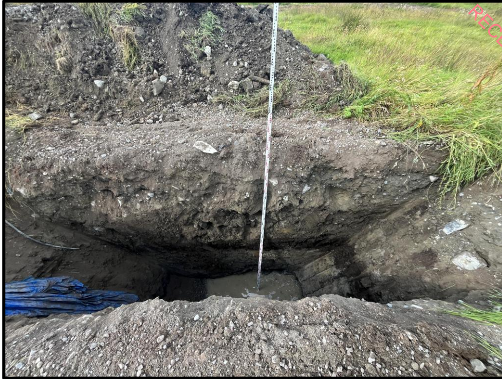
Figure 4: Illustrates the trial hole depth at 3.7m below ground level.
