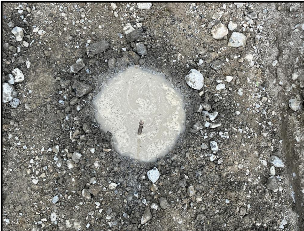
Figure 9: Shows subsurface and surface percolation test carried out.
