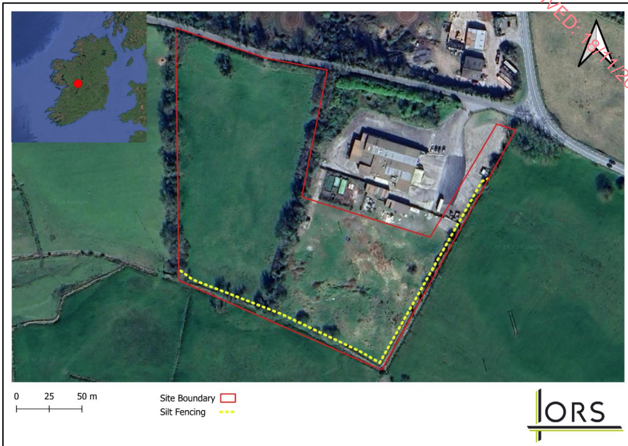
Figure 5.13.1: Proposed site boundary with silt fencing.
