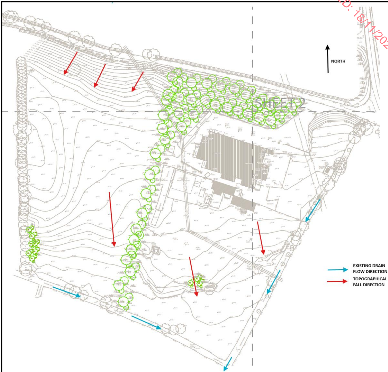
Figure 7.4: Site topography discharging to drainage ditch at the southeast of the site. (Source ORS/J. Weir Land Surveying LTD)
